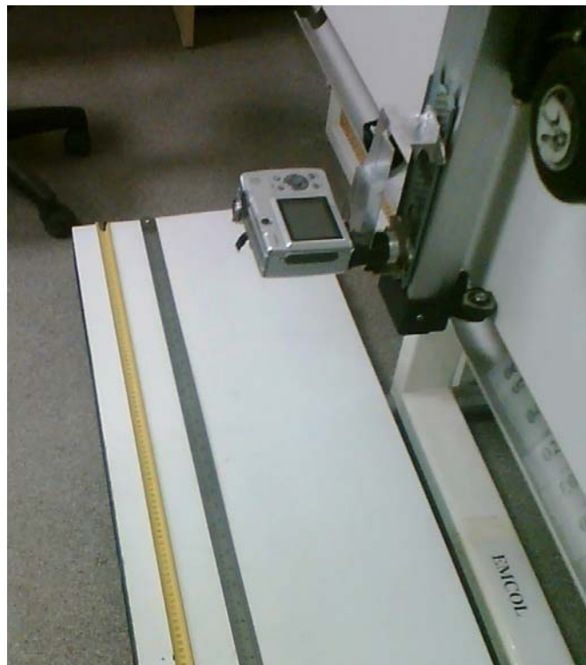
Fig. 14. Core photography set-up with sliding camera on top
