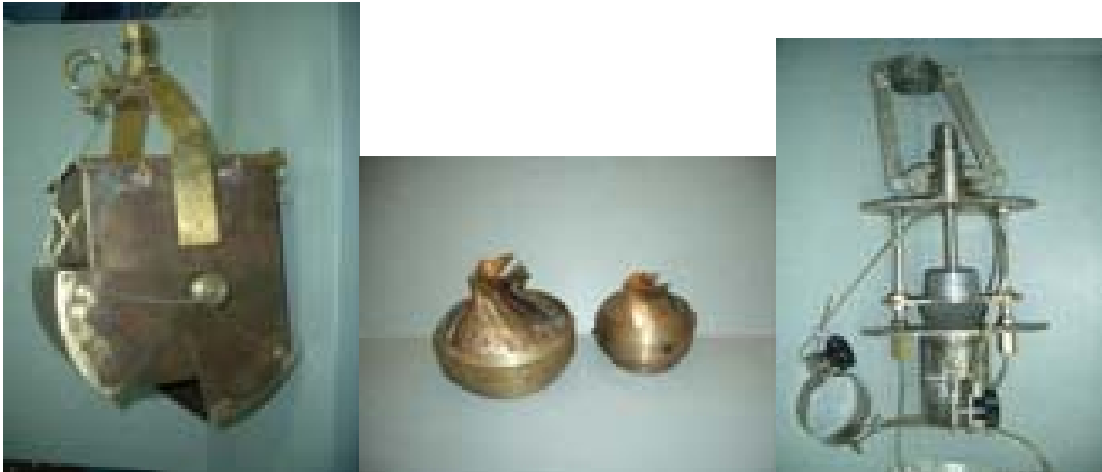
Fig. 8. Some new field sampling equipment manufactured during the second year of the project: grab sampler, core catchers of piston and vibra corers and Kajak Corer (from left to right).
