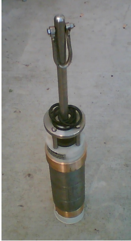
Fig. 9. New Kajak corer manufactured for EMCOL for undisturbed lake sediment coring.
