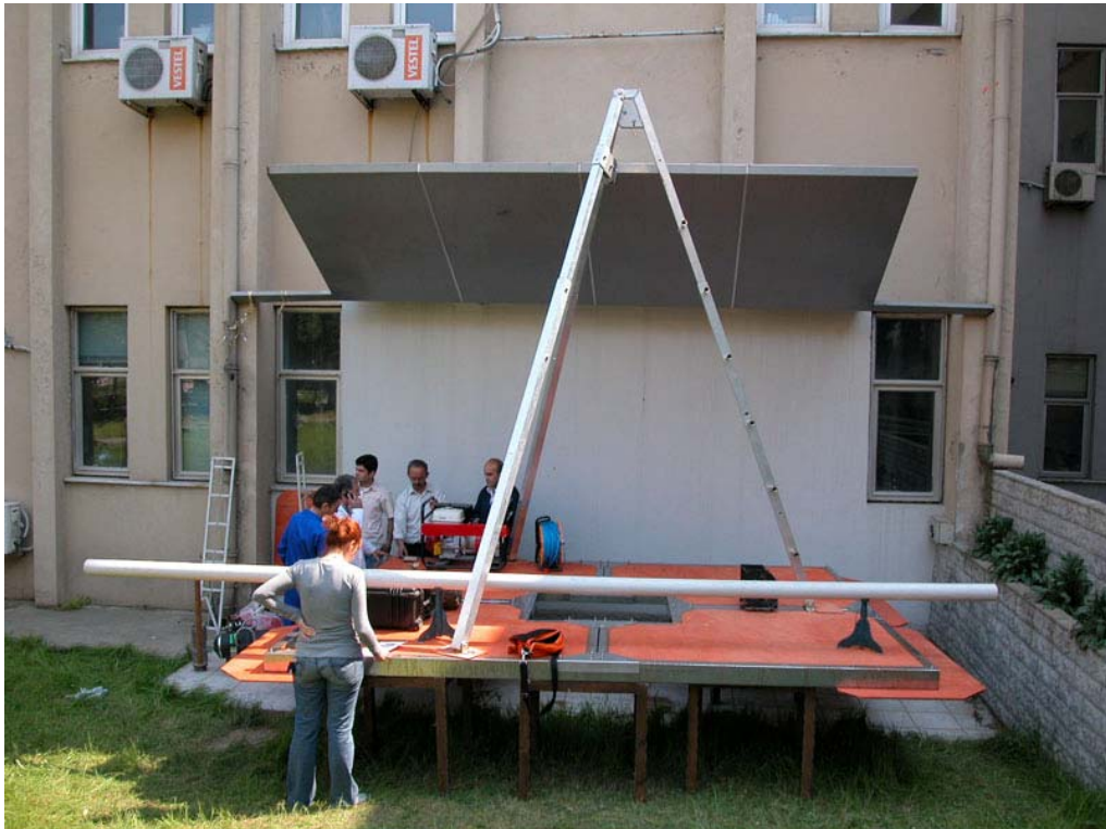
Fig. 11. EMCOL's new platform and tripod for lake sampling
