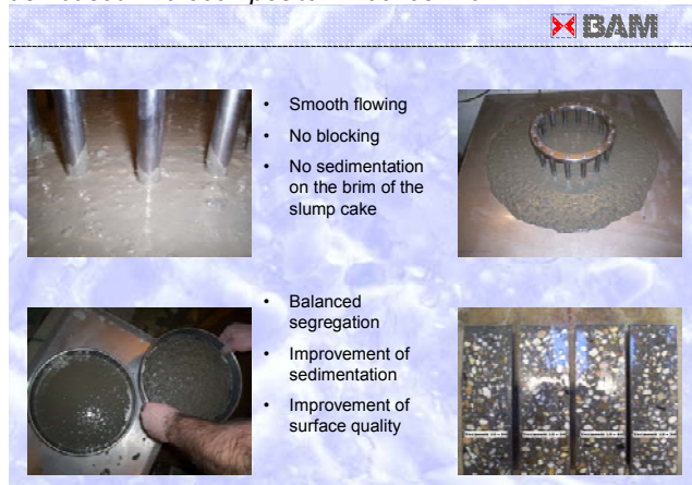
Figure 3. Example on tests with CT-UFFA and SCC.
