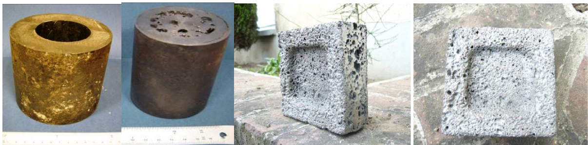
Fig. 5: Iron foam demonstrators made by meltfoaming route
