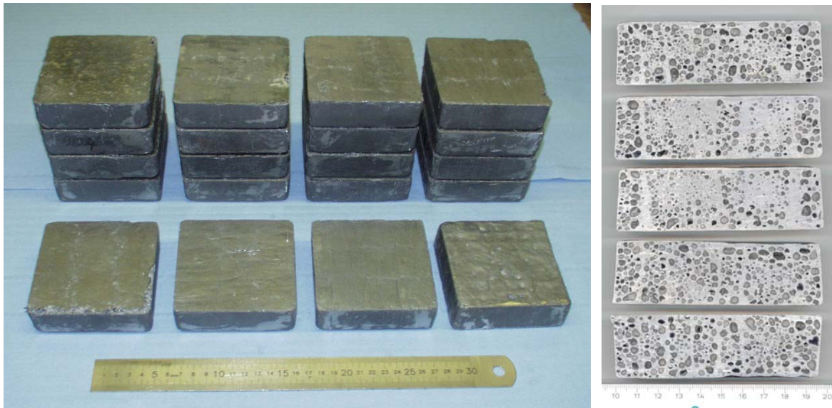
Fig. 2: Cuboid iron foam parts produced in high temperature resistant moulds (left) and cross sections of iron foam part
