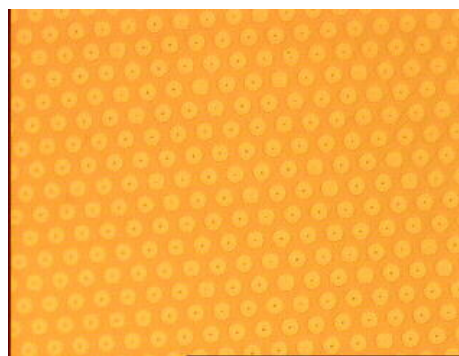
Fig. 17: Snapshot of the surface of a nickel sieve (open pores are identifiable)
