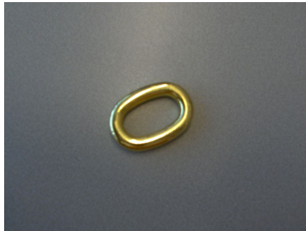
Figure 1: MSA-based white bronze coating on ring with Au topcating
