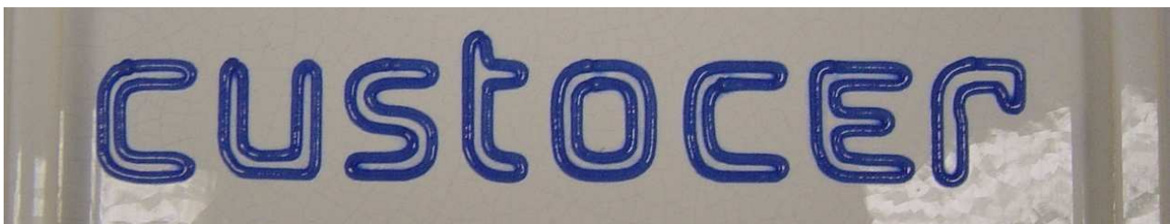
Decorative process using laser cladding techniques. Blue pigment over ceramic tile.
