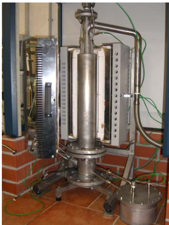
Figure 9: Evaporator and reactor of Teterow sts-plant
