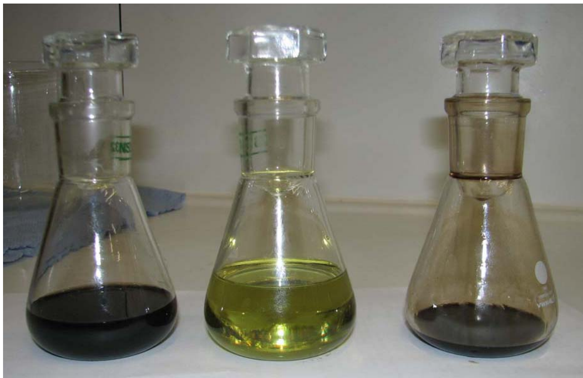
Figure 13: Product sample: crude product (l), purified sample (m) and distillation residue (r)
