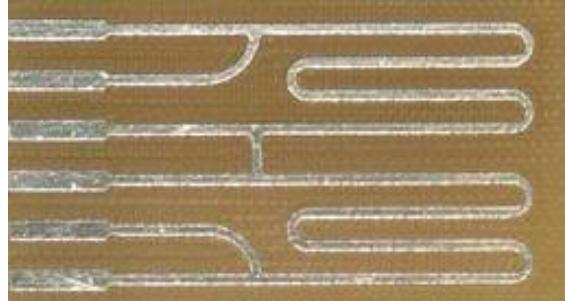
Protection of the reference track against corrosion is provided by a thin organic coating. The coating is transparent to avoid differences caused by heating up of the reference and sensing tracks when irradiated with sun. A polyurethane lacquer was selected from nine tested clear coatings in view of the best wet adhesion and UV stability.
