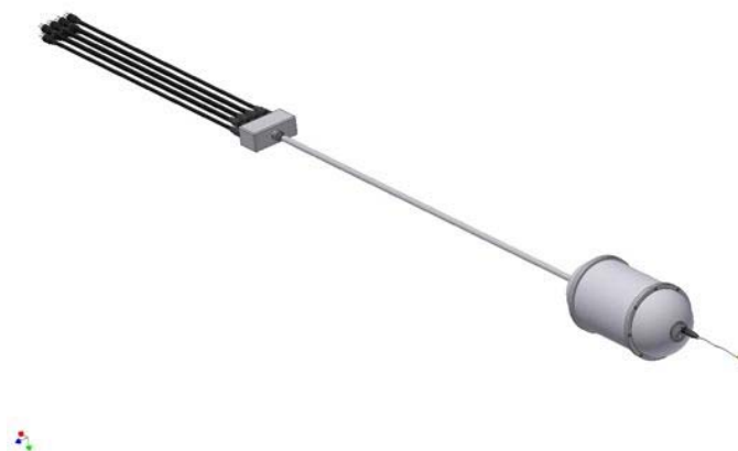
Figure 11. CAD representation of the marinised system showing the electronics enclosure and the tool lead
