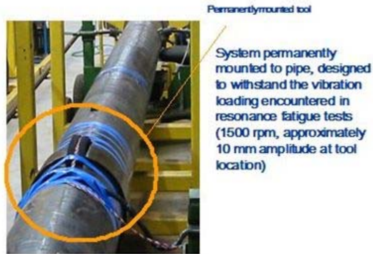
Figure 8. Permanently mounted sensor tool on the riser pipe in the resonance fatigue rig.
