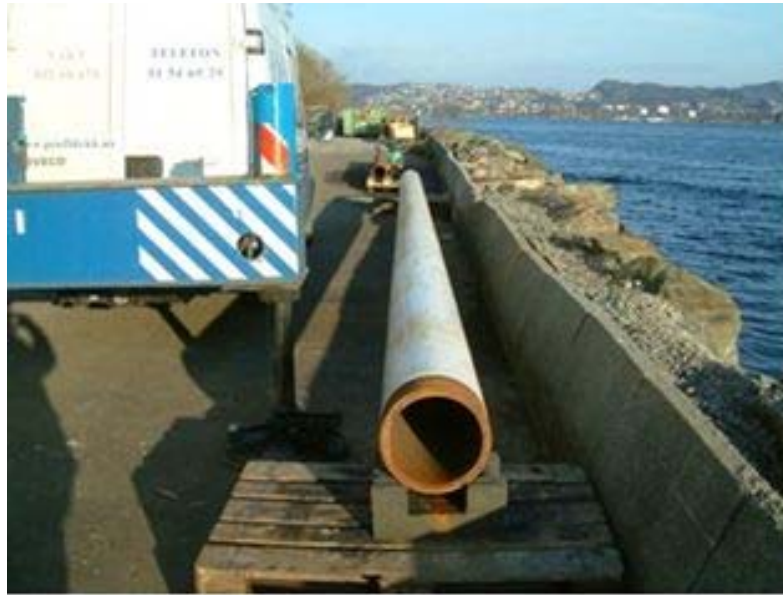
Figure 1. 12" Diameter, 27mm wall polypropylene coated pipe used for the final demonstration
