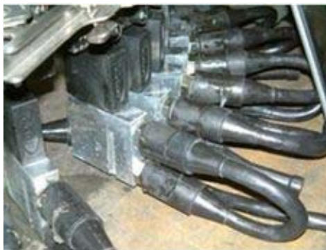
Figure 13. Detail of the sub-sea bracelet tool, showing the underwater connectors
