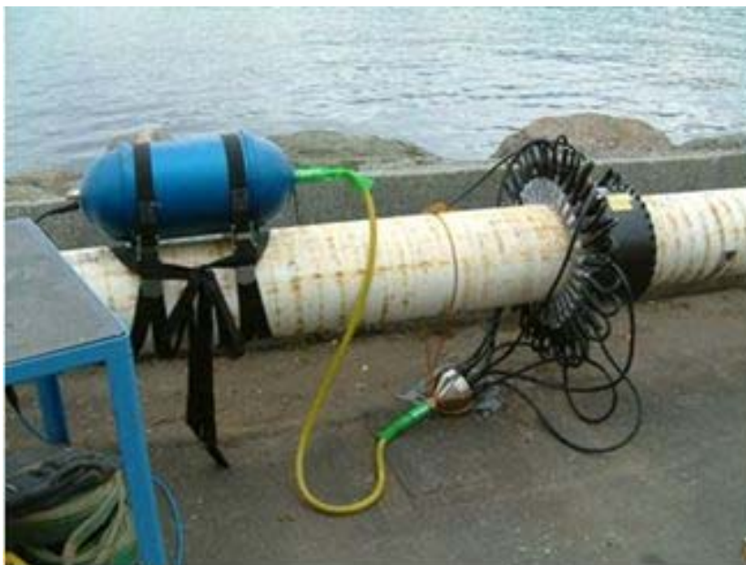
Figure 15. Prototype sub-sea system mounted on the coated riser pipe
