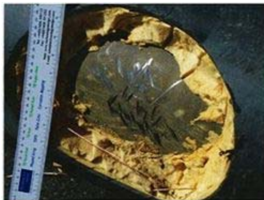
Figure 7. Defect in coated pipe, width 80mm, length 92mm, reduced area 5.8%
