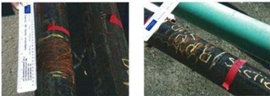
Figure 6. Irregular defects in bare pipe, made by a series of grinding marks
