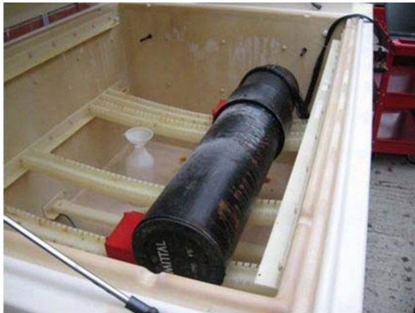
Figure 9. Specimen mounted in the salt spray chamber. The lead for conducting the in-situ ultrasonic tests may be clearly seen
