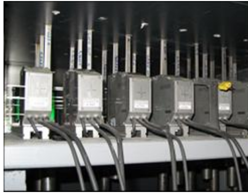
Figure 6.23. Array of 28 samples and optical micrometers, under the furnace.
