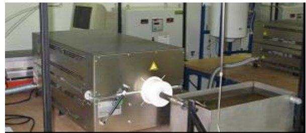
Figure 6.34. Tube furnaces, holding a single atmospheric reactor.
