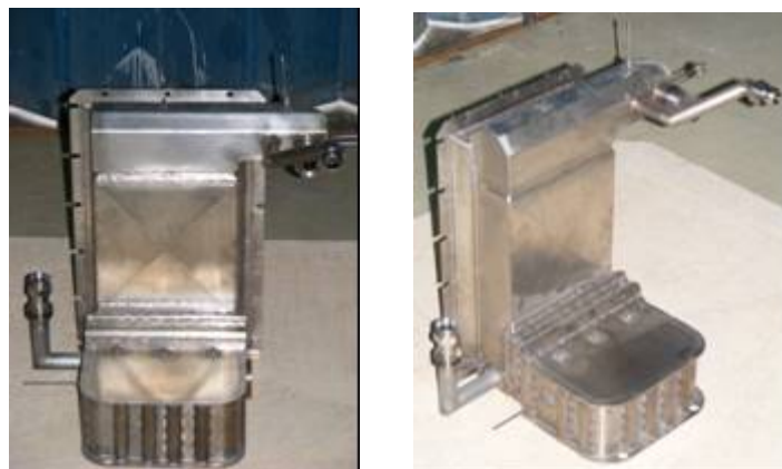
Figure 6.8. 15kWe Stack Block Rig Heat Exchanger assembly.
