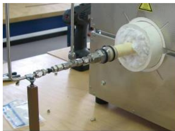
Figure 6.31. Reactor inlet, showing A: press. water feed; B: reactor for atmospheric tests.
