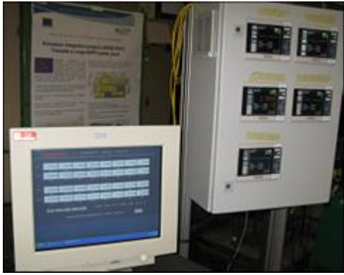
Figure 6.22. Data acquisition system for medium precision creep measurements.
