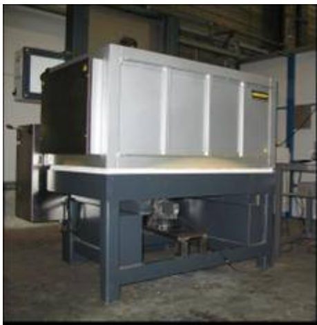
Figure 6.20. Furnace for medium-precision creep measurements.
