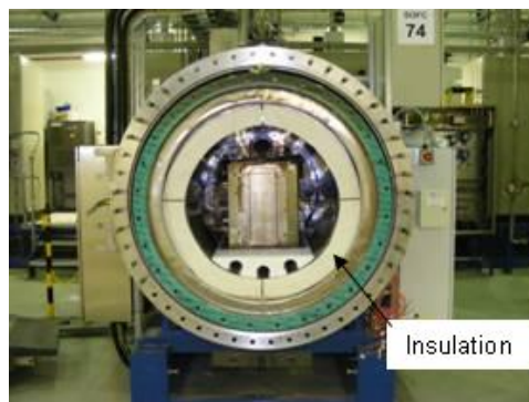
Figure 6.50. 15kWe Stack Block Rig – Insulation.
