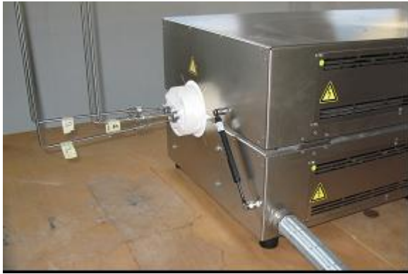
Figure 6.35. Tube furnace, showing the inlet tubing for gas and water flows.
