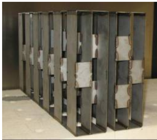
Figure 6.21. Creep-resistant chassis for medium-precision creep measurements.
