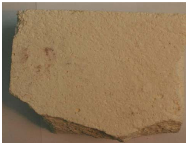
Figure 6.51. Failed insulation sample after high temperature compression.
