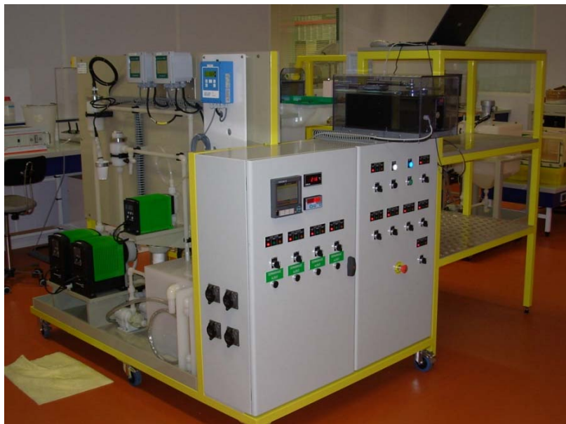
Fig. 48: 30 \times 60 \text{ cm}^2 electrodeposition reactor
