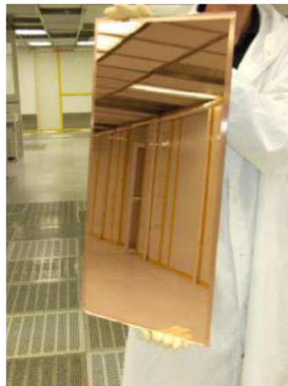
Fig. 42: Photography of a 30x60 cm 2 electrodeposited layer of Cu/Mo/glass with 6% of standard deviation.
