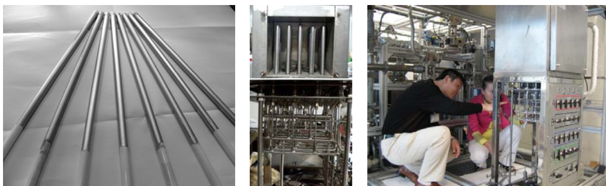
Figure 1.5: Prototype scale membrane separation unit and integration into the Liquid Fuel Test Unit at DLR for testing.
