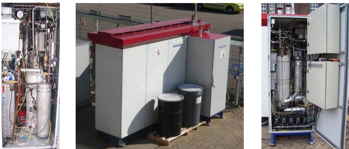
Figure 1.6: NEMESIS proof-of-principle prototype (middle) with Fuel Preparation Module (right) and Hydrogen Generation Module (left)
