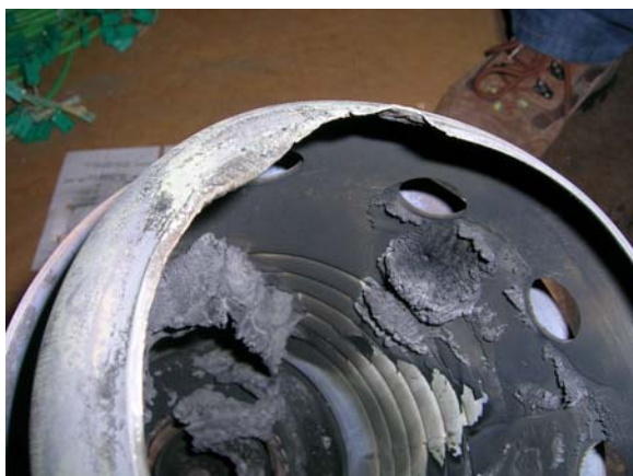
Figure 53 Damaged flame tube
