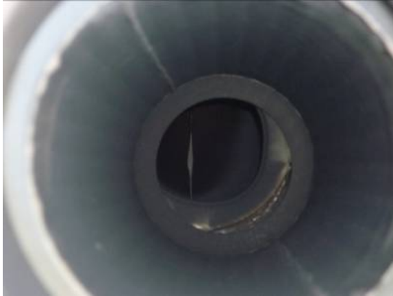
Figure 55 Eccentric position of external flame tube
