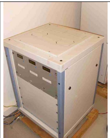
Figure 8 – Complete lithium based inverter with instrumentation
