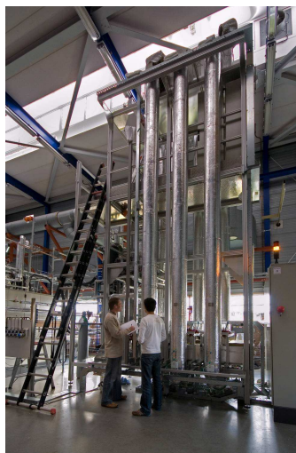
Figure 1.9 SEWGS Multicolumn unit
