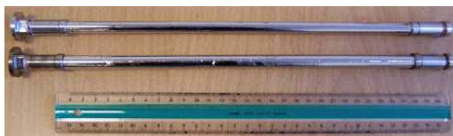
Figure 1.6: 2 µm thick Pd/alloy membranes on porous stainless steel (PSS®) support produced by SINTEF
