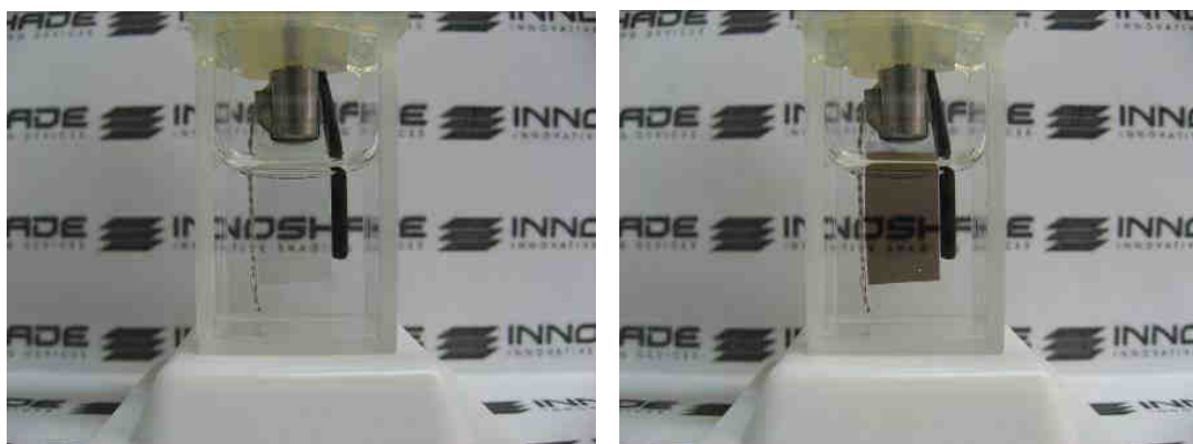
Figure 4. Bleached (left) and coloured (right) states of the polyISO-7 colour modifier layer. Photos: R. Ruffo/Università degli Studi di Milano-Bicocca.
