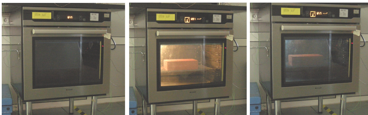
Figure 19. Household oven prototype with included INNOSHADE EC film for energy consumption modelling. Left: dark state – internal light off, middle: clear state – internal light on, right: dark state – internal light on. Photos: O. Ersoy/ARCELIK.
