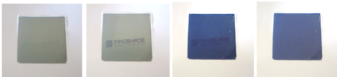
Figure 7. Optical states of a PDLC-EC tandem device: hazy-colourless (PDLC off, EC 2.0 V / blue curve), clear-colourless (PDLC on, EC 2.0 V / green curve), clear-blue (PDLC on, EC -2.0 V / red curve), and hazy blue state (PDLC off, EC -2.0 V / black curve). Photos: J. Palenzuela/CIDETEC.
