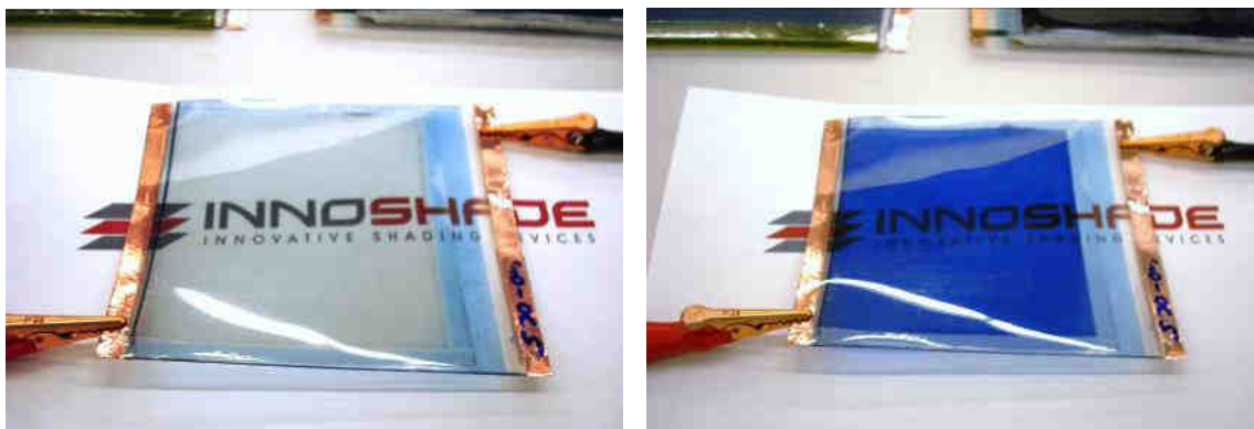
Figure 8. Flexible plastic-based electrochromic device. Left: Bleached state, +1.5 V; Right: darkened state, -1.5 V. Photos: U. Posset/Fraunhofer ISC.
