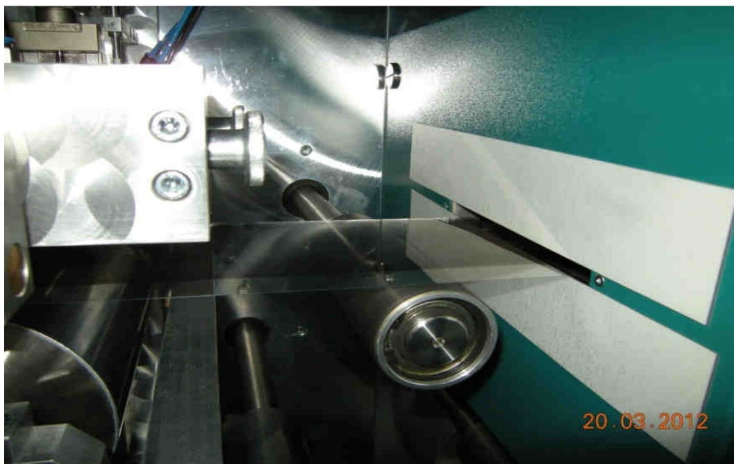
Figure 5. Application of a \text{Ni}_{1-x}\text{O} pigment suspension on PET-ITO film on a COATEMA Smartcoater. Photo: M. Mohor/National Institute of Chemistry Ljubljana.
