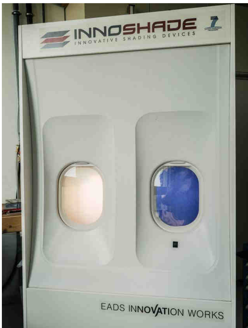
Figure 17. Demonstrator of an Airbus A320 cabin wall equipped with an INNOSHADE EC device. Photo: H. Fietzek/EADS.
