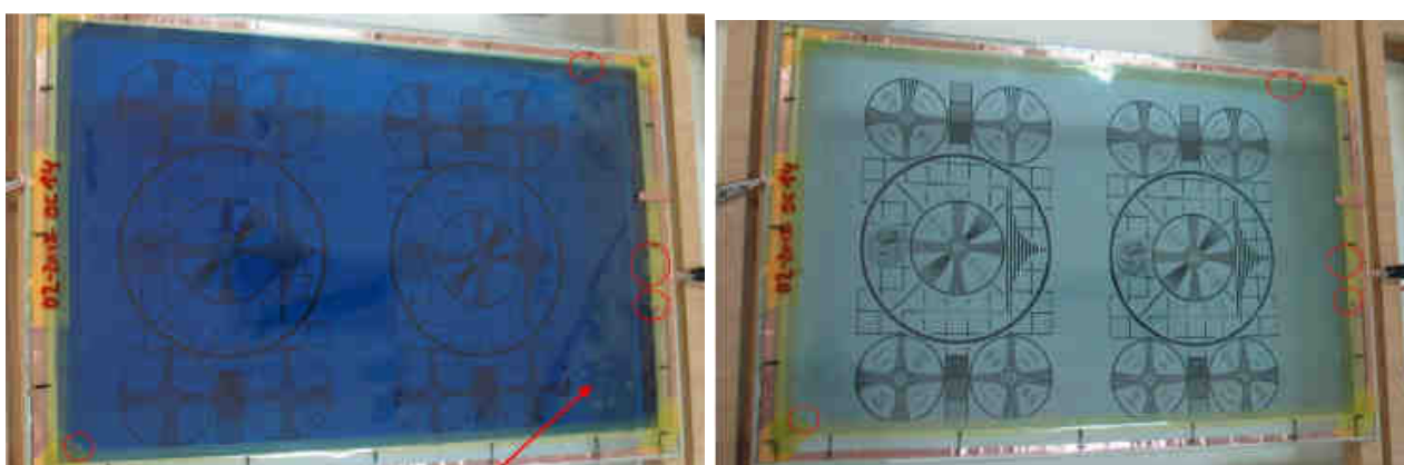
Figure 9. Left: Coloured state, right: bleached state of an INNOSHADE appliance door demonstrator (size A3+). Photos: B. Kralj/ GORENJE.
