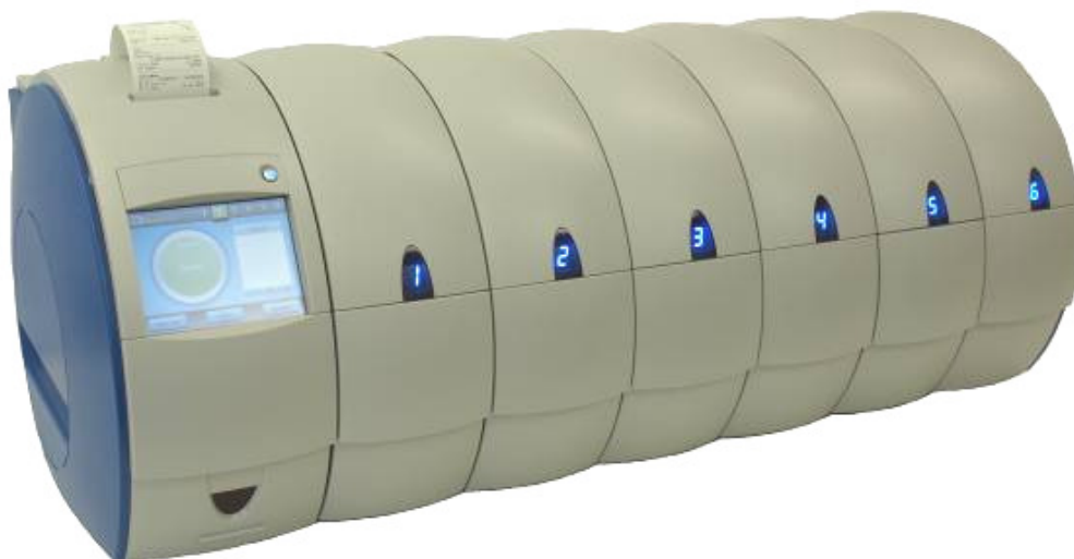
Fig 24. Enigma@ML CM and PM sub-system integration to a 6 module, higher-throughput diagnostic system.
