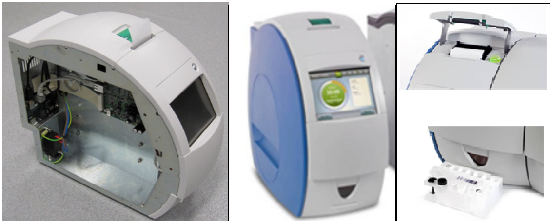
Fig 9. 'A1' early prototype CM (left), 'A3' production-ready prototype CM (centre), thermal printer (top right), external bar-code reader (bottom right).
