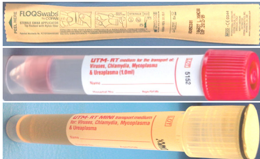
Fig 2. Selection of COPAN CE-marked nasal swab (top), standard COPAN UTM-RT sample tube (middle) modified COPAN UTM-RT with RANGER ML compatible lid modifications (bottom).
