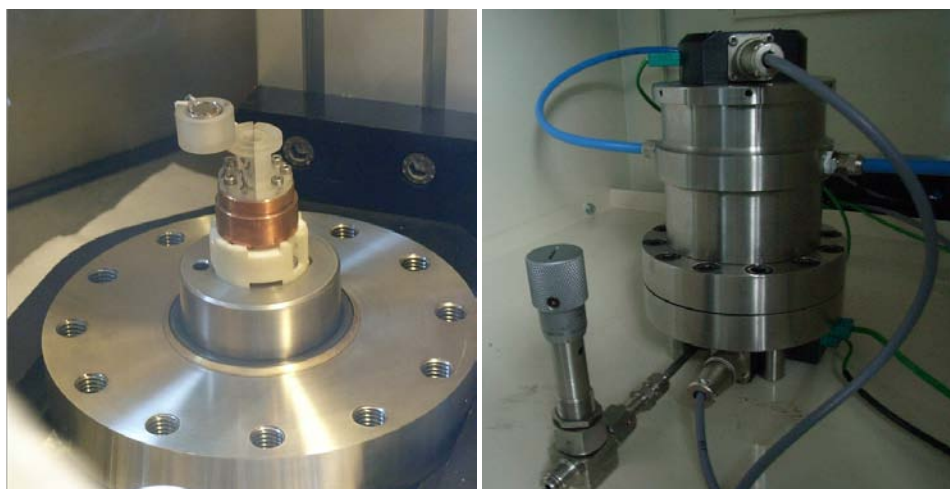
Figure 25: Pictures of the sample holder for thermal conductivity measurements and the thermalized vessel.
