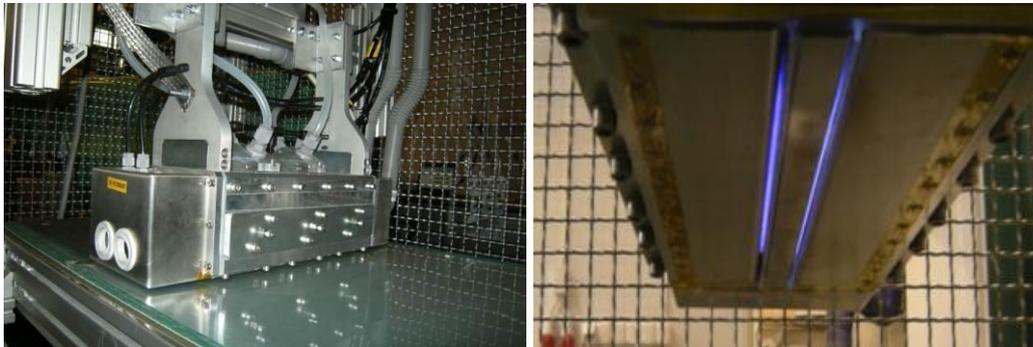
**Figure 1 200 mm wide lab scale plasma system installed at VTT for process development.**
