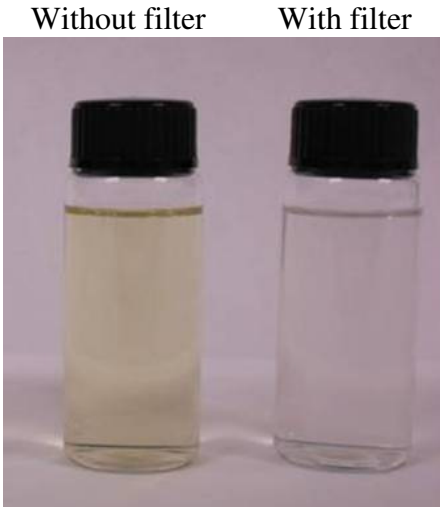
Figure 5: Effect of filter on tar recovered.
