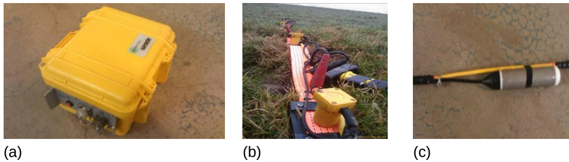
Figure 4 - (a) Vertical component geophones of 10 Hz central frequency (Geospace), (b) vertical component geophones of 100 Hz central frequency (Mark Products), (c) tractable gambles of 10 Hz central frequency (Mark Products).
