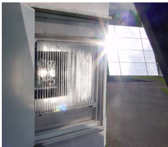
Figure 5: Solar \text{H}_2\text{SO}_4 decomposer receiver-reaction in operation in a solar furnace.
