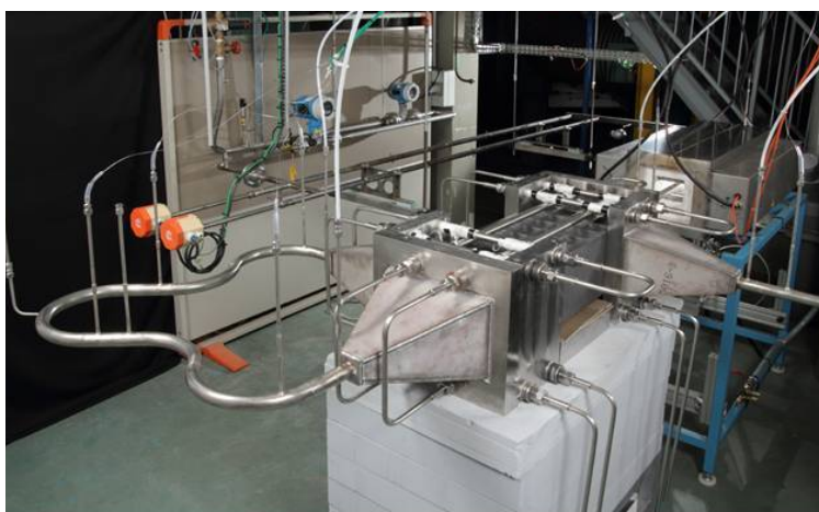
Figure 3: SiC prototype on the thermal test rig (before being thermally insulated).
