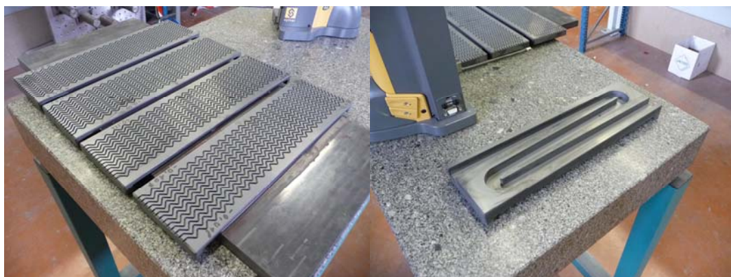
Figure 2: SiC channelled plates of the prototype: heat source plates (left) and a reaction plate with one large meandering channel (right).
