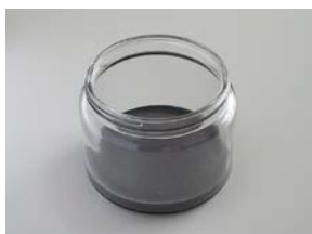
Figure 1. The contaminant trap glass. A composite of the silicone PDMS and activated carbon is cast into the bottom of a glass, where it acts as an infinite diffusion sink for polycyclic aromatic hydrocarbons.
