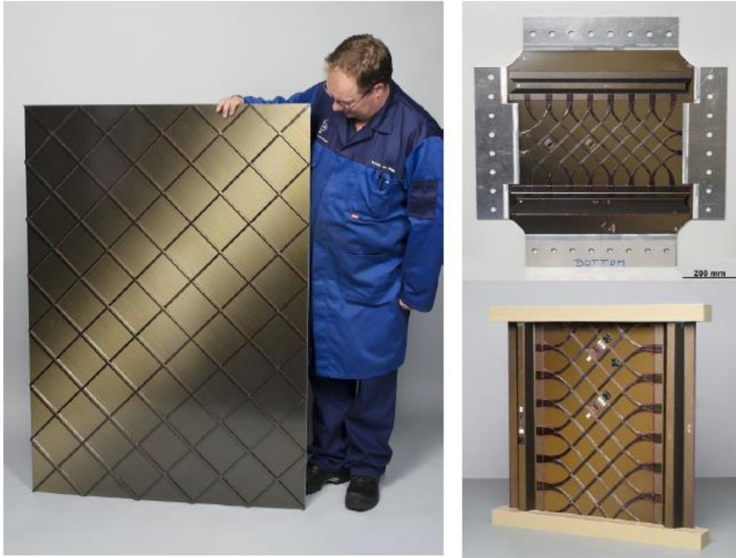
Figure 15: High grid, low grid shear and low grid compression panels as manufactured
