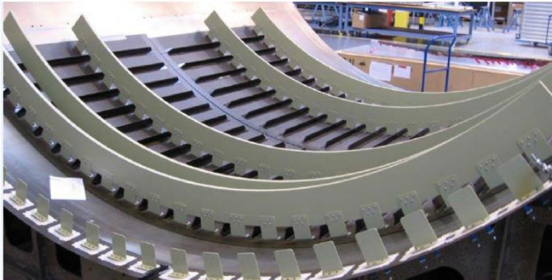
Figure 17: Assembly of the external butt strap test specimens (1 AI-D)
