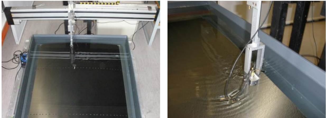
Figure 34: Test setup for ultra-sonic inspection of the stiffened panels
