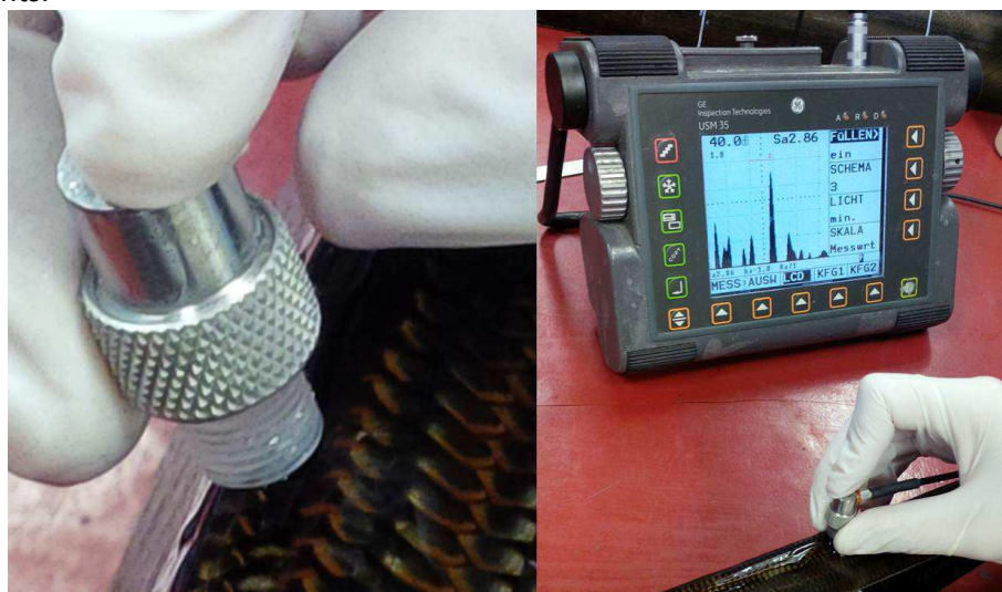
Figure 28: US inspection using A-Scan
