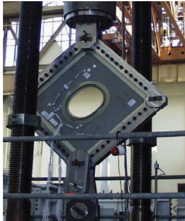
Figure 46: RTM window frame (56 TAI) co-bonded on a skin panel for testing at partner (25) IMA
