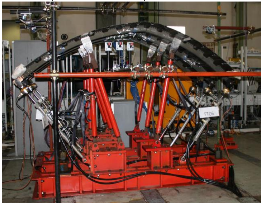
Figure 45: Panel bending testing at partners 63 ALA and 25 IMA
