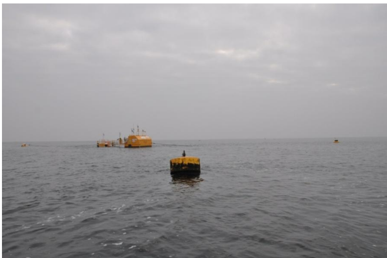
Figure 3.9: OE Buoy installed at Galway Bay Intermediate Wave Energy Test Site
