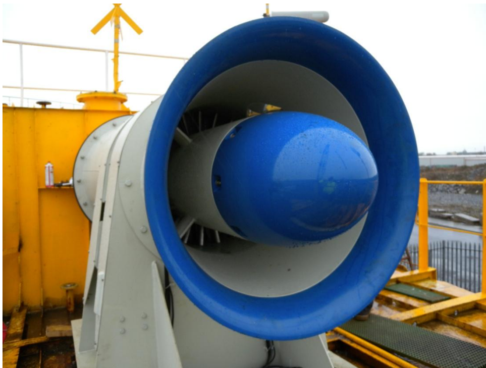
Figure 3.14: CORES Impulse Turbine with Moveable Guide Vanes
