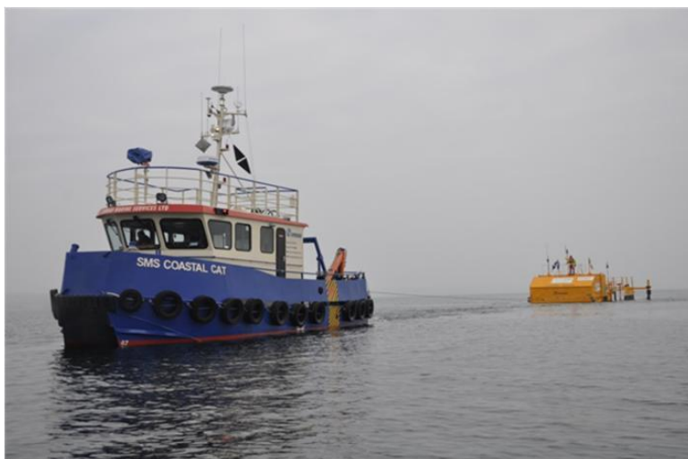
Figure 3.8: OE Buoy being towed to Galway Bay Intermediate Wave Energy Test Site
