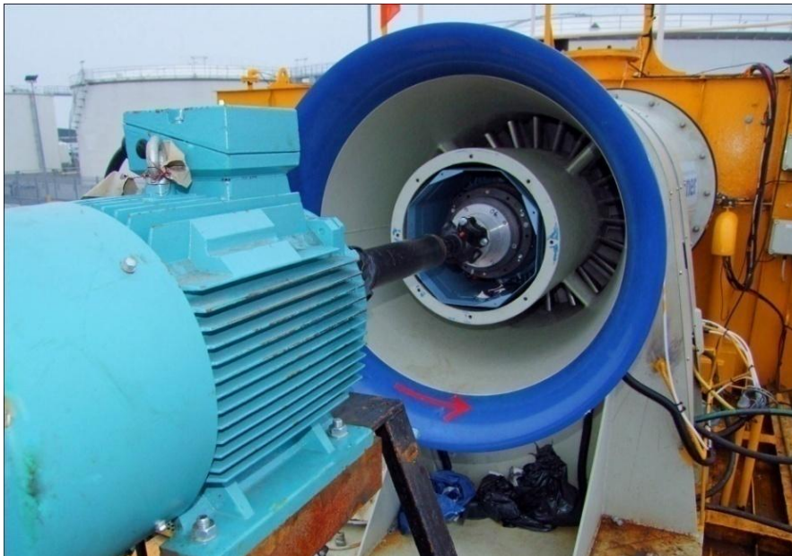
Figure 3.3: Testing of air turbine by manually spinning
