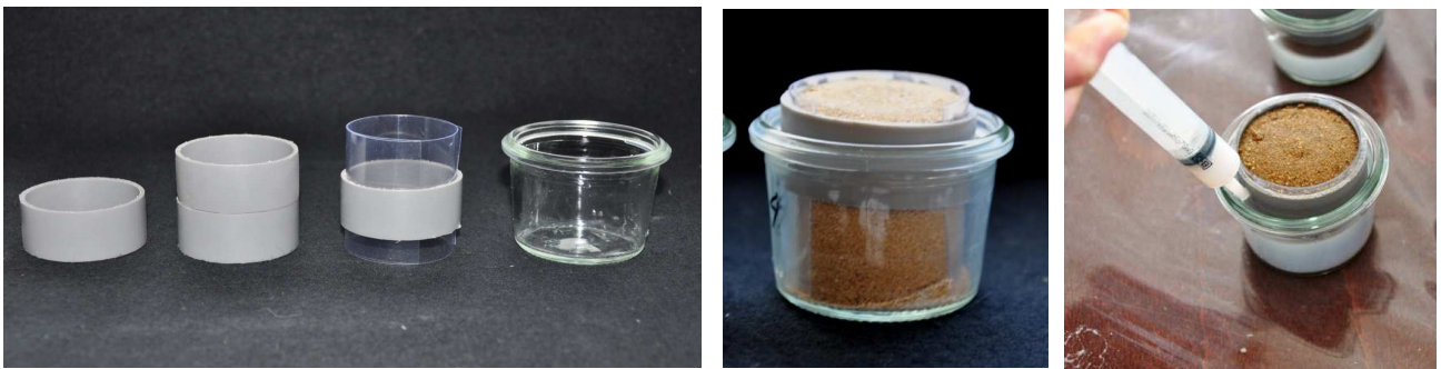
Fig. 6-8 Test kit to characterise the consolidation of loose aggregates by capillary suction (Strotmann & Partner)
