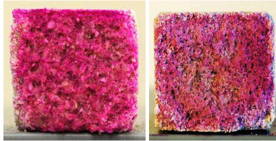
Fig. 23 Distribution of calcium hydroxide nano-particles in mortar samples after 24 hours indicated by the red colour of the indicator phenolphthalein (University of Fine Arts, Dresden)
