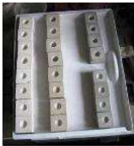
Fig. 14 Drill holes in intact stone after saturation with CaLoSiL ® (Restauro, Torun)
