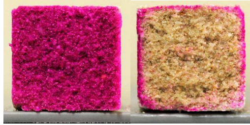
Fig. 22 Distribution of calcium hydroxide nano-particles in mortar samples indicated by the red colour of the indicator phenolphthalein (University of Fine Arts, Dresden)
