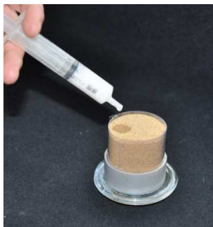
Fig. 6-8 Test kit to characterise the consolidation of loose aggregates by capillary suction (Strotmann & Partner)
