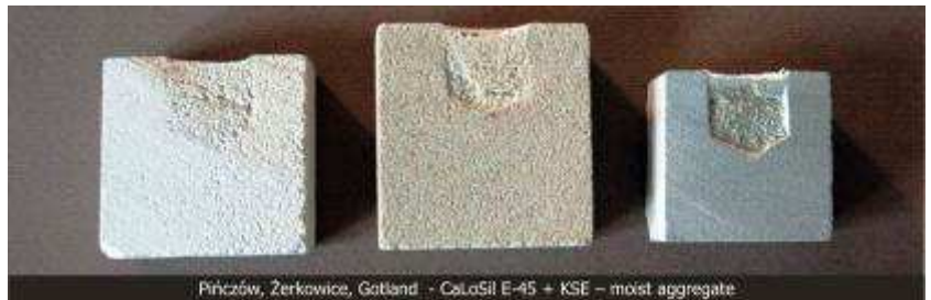
Fig. 15 Cross sections of the samples after consolidation (Restauro, Torun)
