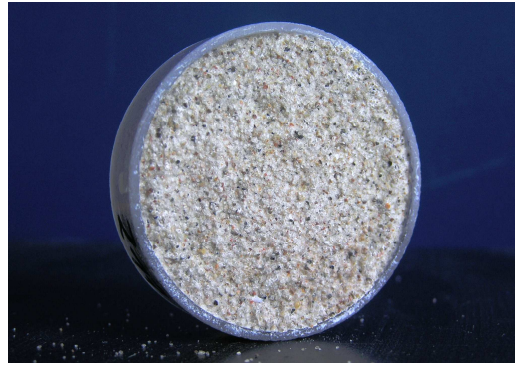
Fig. 26 Loose sand particles consolidated by combined treatment with CaLoSiL ® E-25 and Funcosil 300 (producer: Remmers, Germany), (IBZ-Freiberg)
