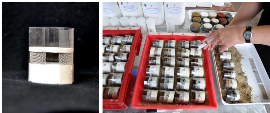
Fig. 10, 11 Test kit to characterise the consolidation of loose aggregates between intact stone / mortar (Strotmann & Partner)
