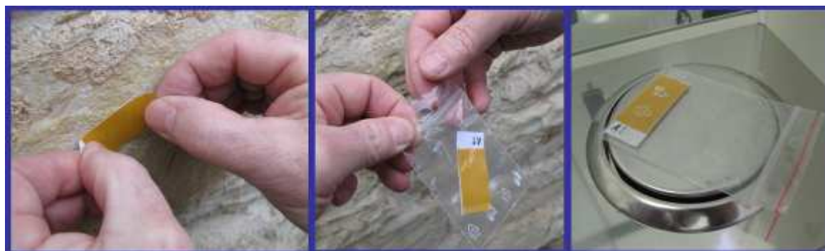
Fig. 37 Peeling test"- Experimental procedure (ITAM AS CR, v. v. i, Prague)
