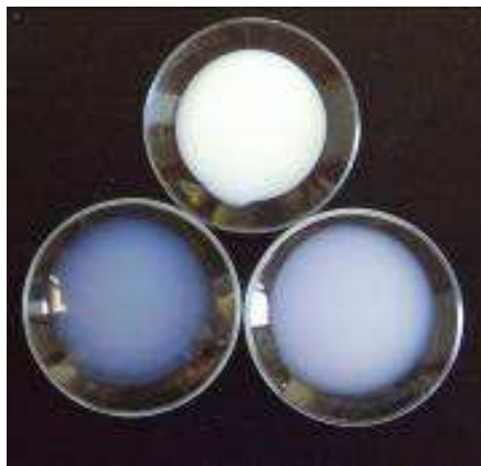
Fig. 3 Different types of calcium hydroxide nano-sols (IBZ-Freiberg)
