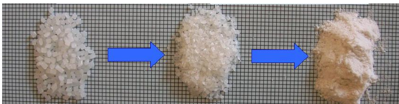
Fig pellets after conventional polymer milling and HEBM process
