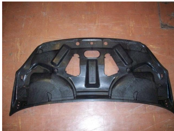
Figure 23. Automotive bonnet containing CNTs manufactured in the project.
