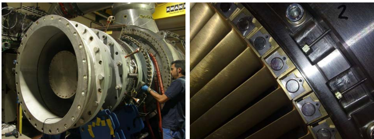
Figure 20. CTA high speed wind-tunnel (left) and close-up of the rotor blade tip-shroud with the rotating magnets and blade tip timing optical probes (right)
