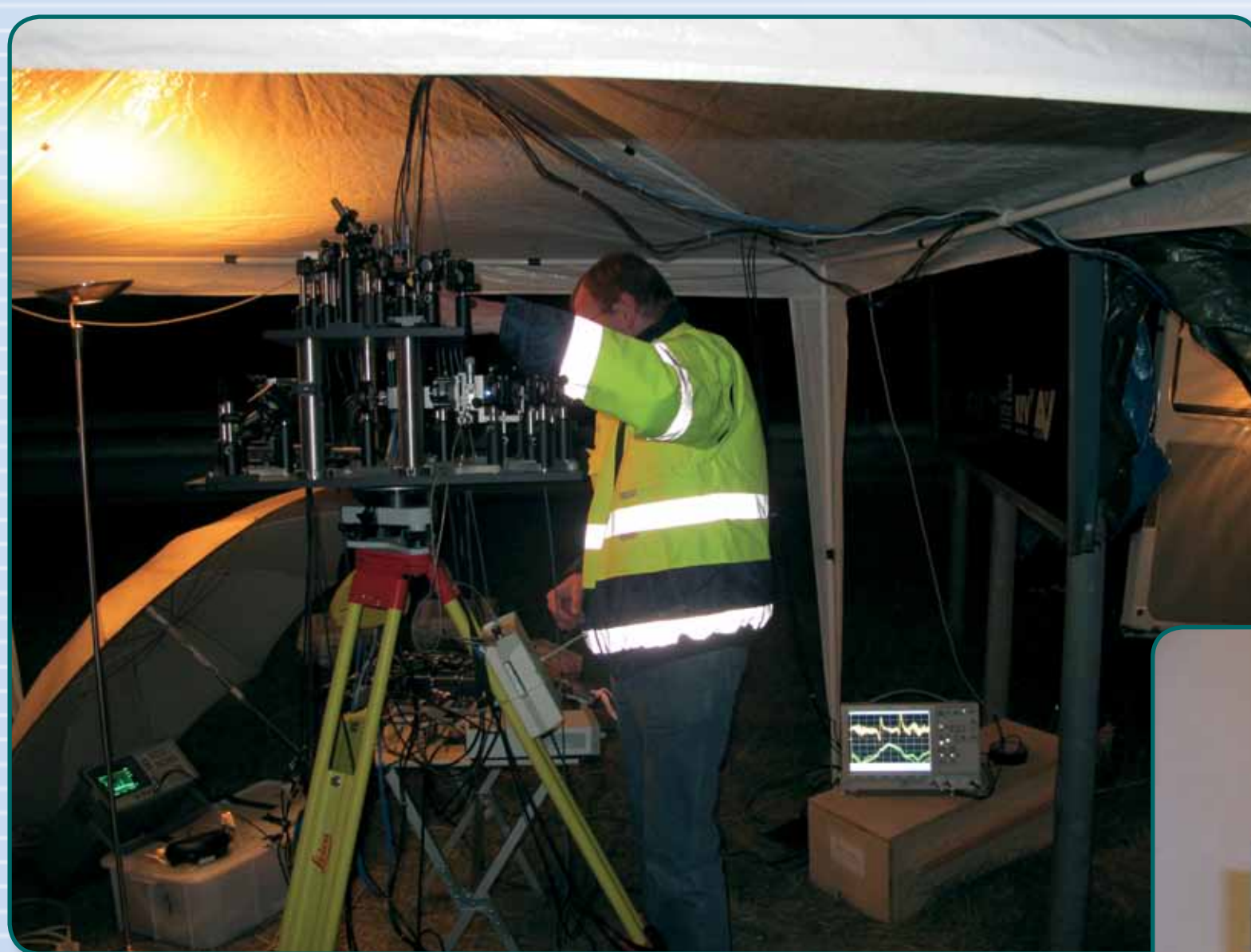
▶ VSL laser interferometer used for validation of pulse to pulse interferometry and femtosecond based telemeter.
