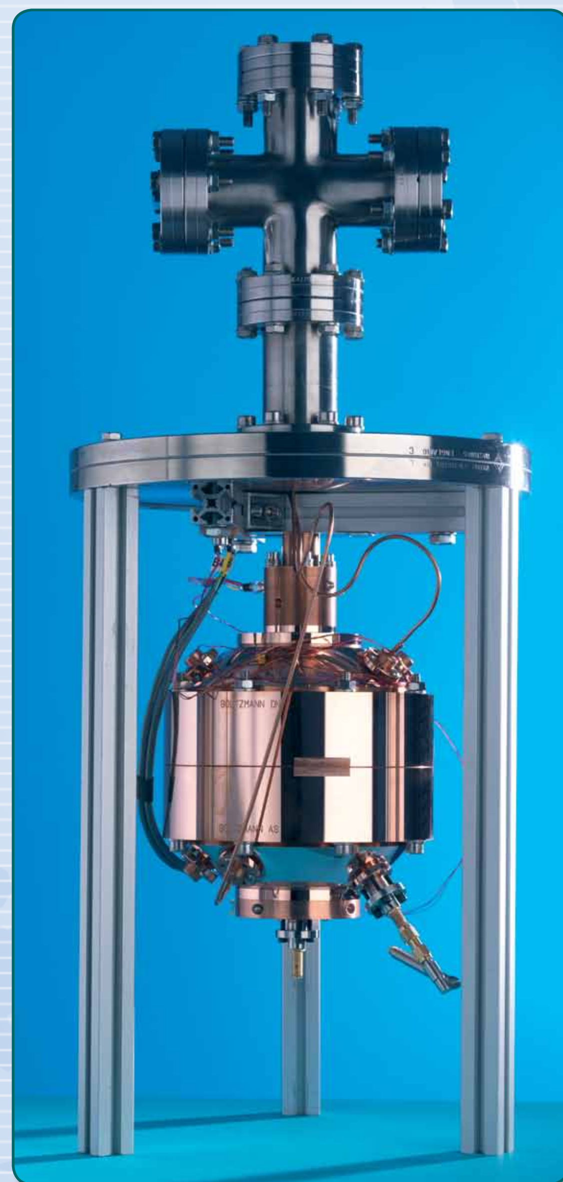
AGT Cell - Spherical resonator for acoustic gas thermometry (AGT).
