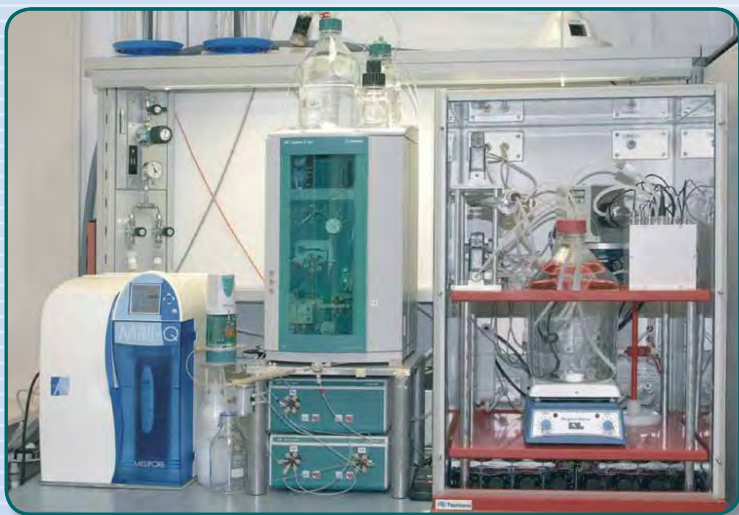
Photo of the closed loop measurement setup for conductivity measurements in purified water with controlled electrolytic contamination: the temperature control box can be seen on the right hand side, containing the conductivity measurement cell, the pump and the contamination vessel; the right hand side shows the purification system for highly purified water, the dosage unit for contamination and the ion chromatograph.
