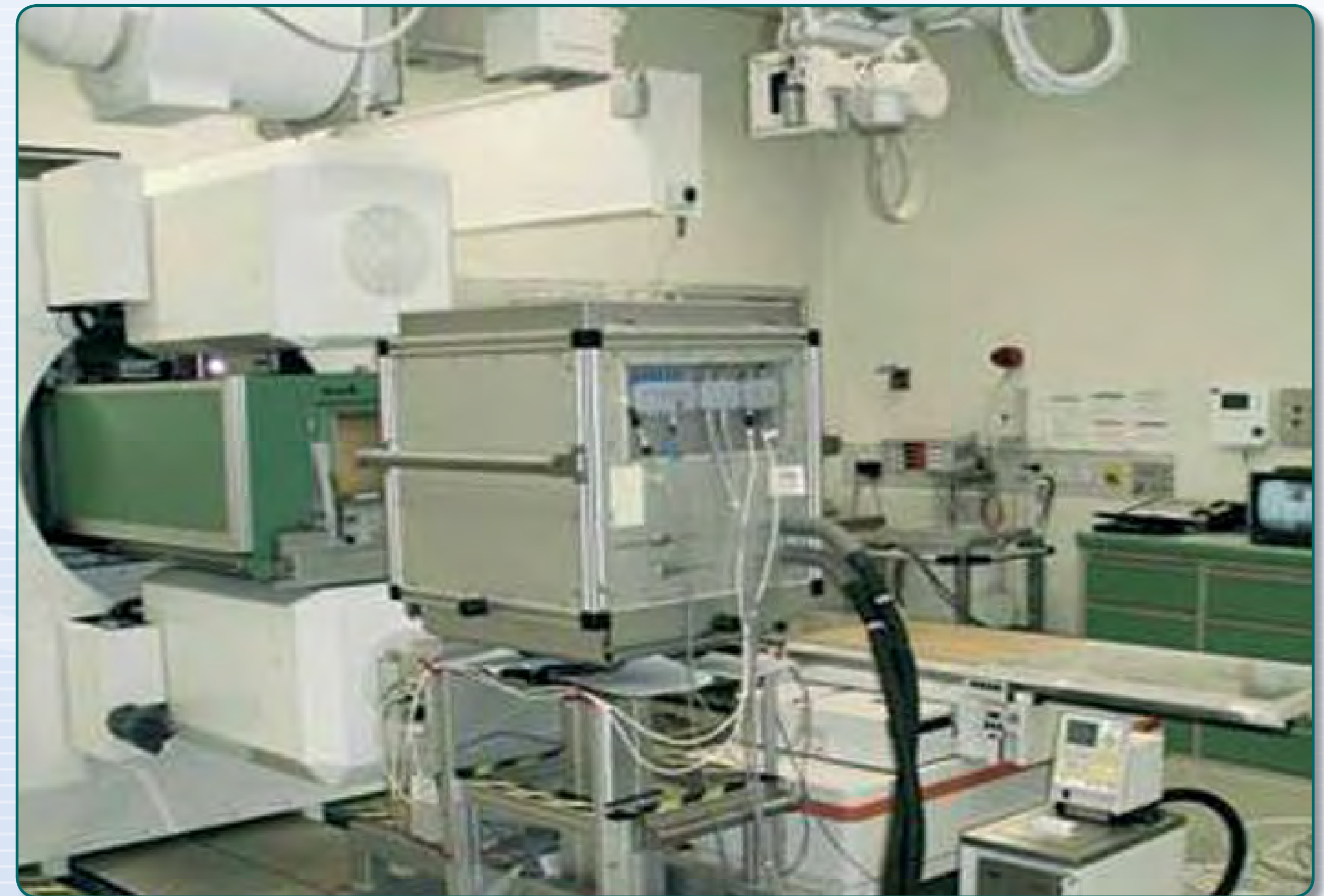
Transportable water calorimeter (PTB) at the 12C beam line at GSI in Darmstadt, Germany.
