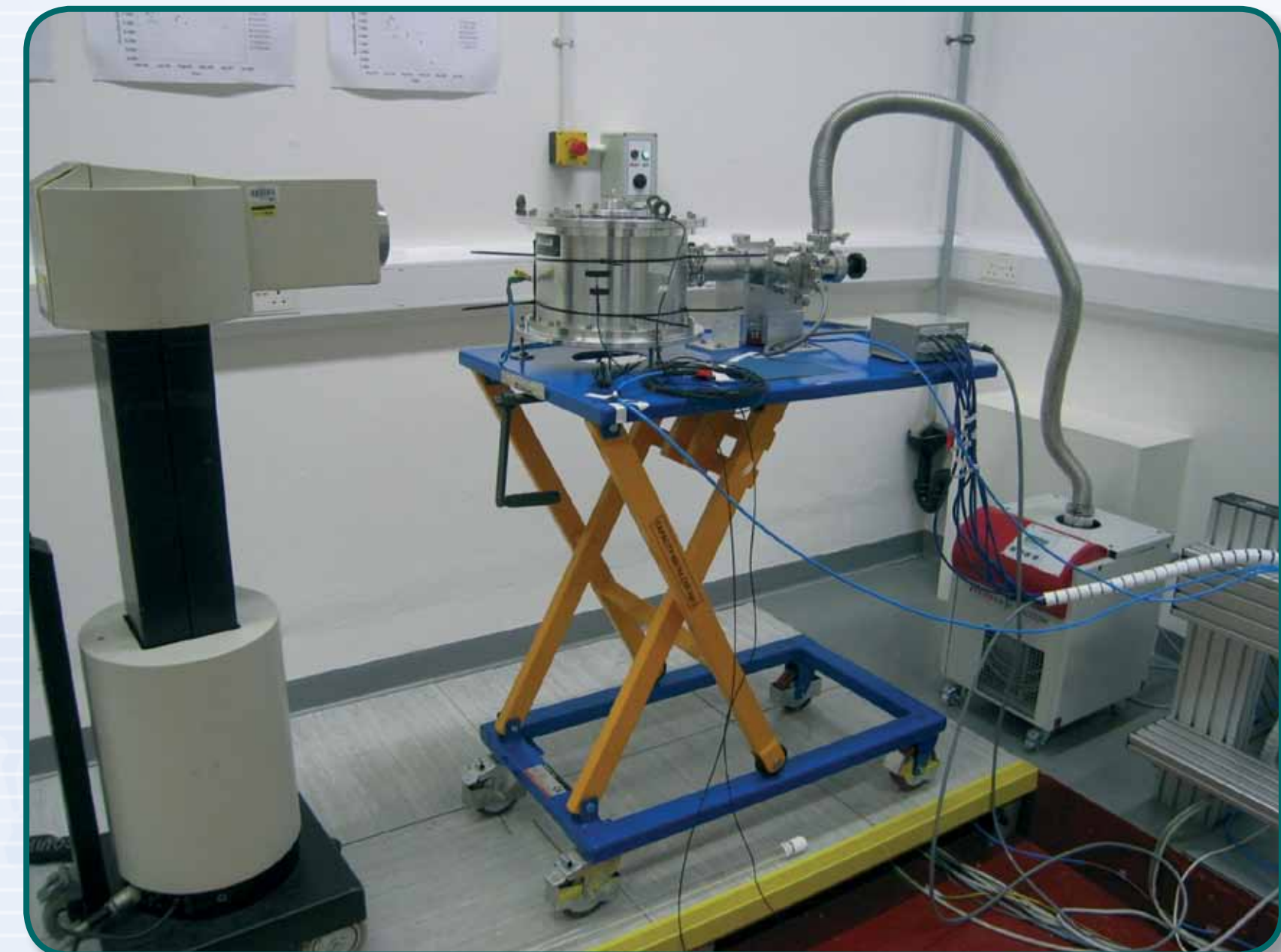
Graphite calorimeter developed by NPL with Nucletron microSelection Classic afterloader. The treatment unit is connected to the calorimeter via a transfer tube.
