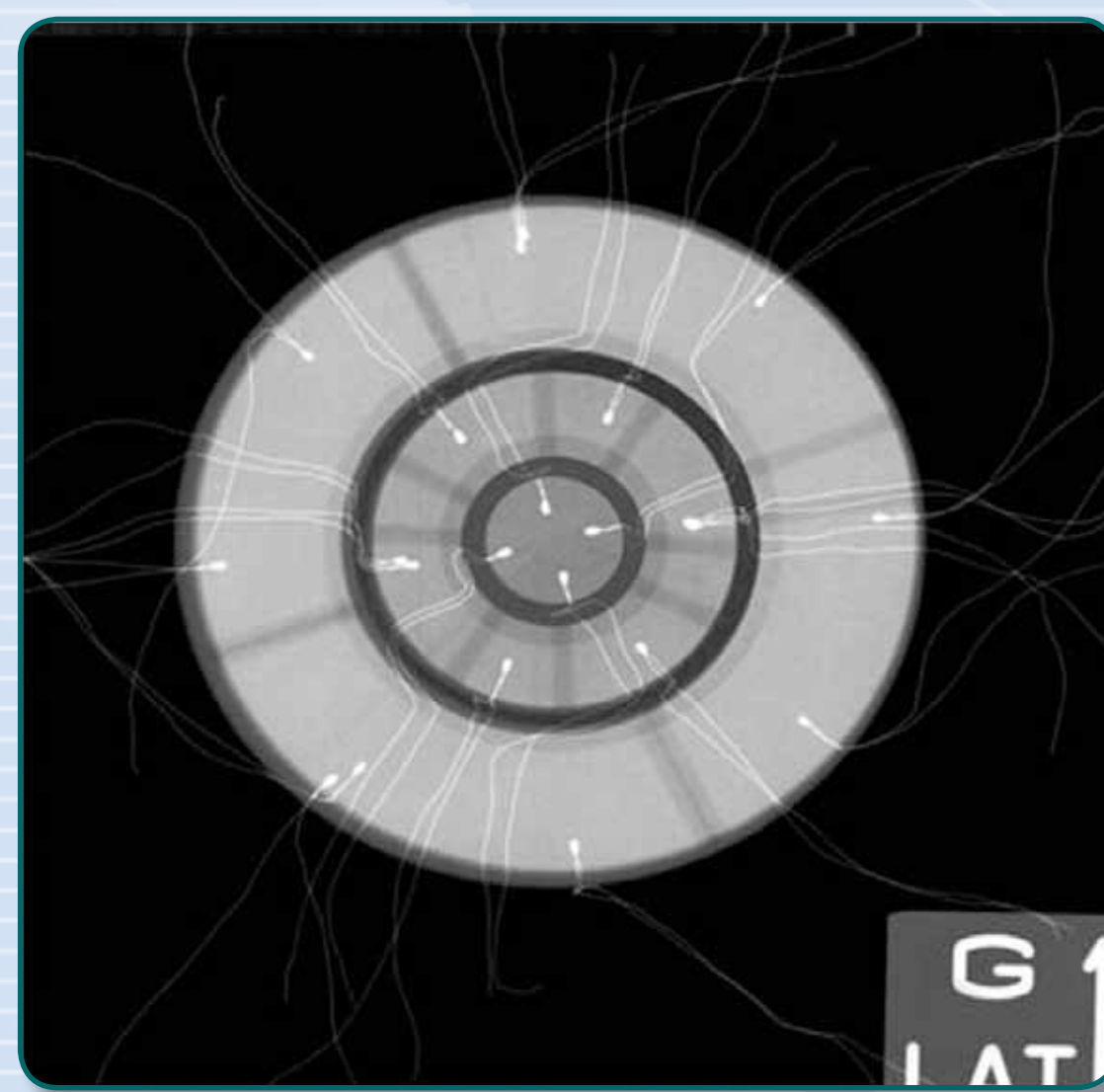
Radiography of the core of the graphite calorimeter (LNHB) for the realisation of D_w in photon fields with a size down to 2 cm x 2 cm.
