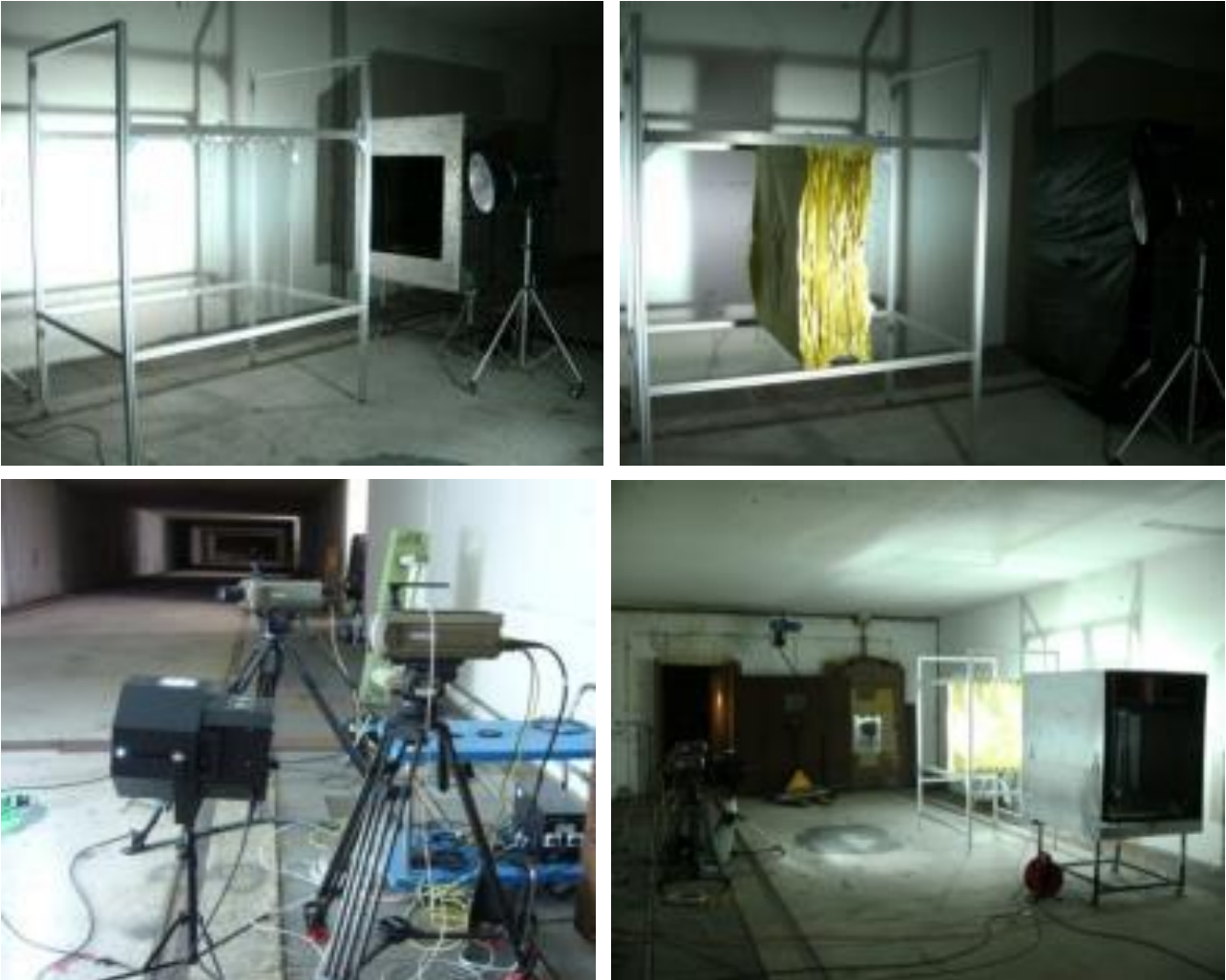
Figure 10: Experimental set-up at Fh-ICT firing range, including testing racks and high speed cameras and infrared light barrier to detect the bullet velocity
