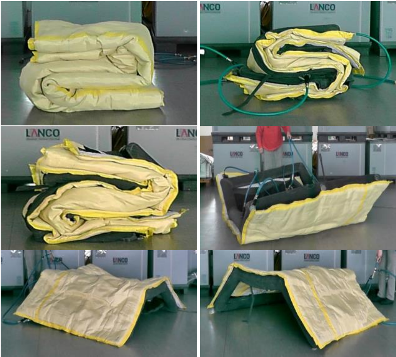
Figure 33: Unfolding of a ballistic pack by inflation by compressed air
