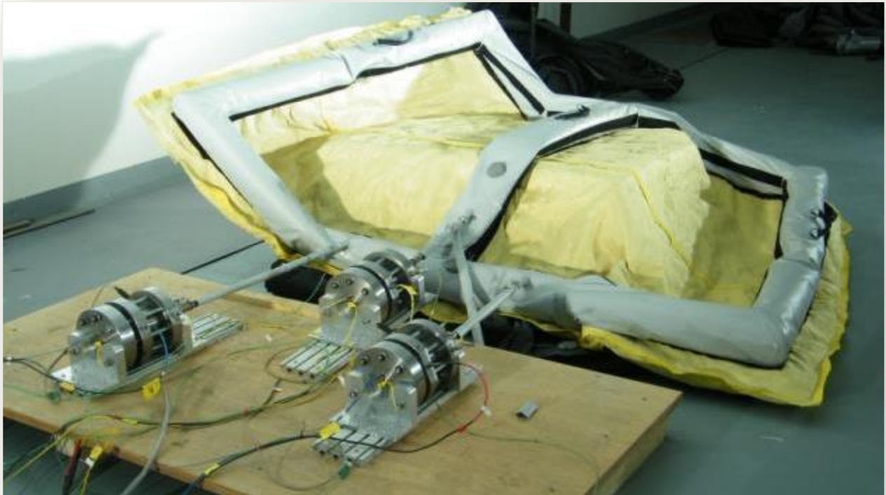
Figure 34: Three cold gas generators adapted to inflate the frame structure for unfolding of a ballistic pack
