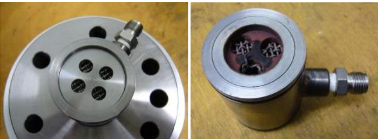
Figure 25: Photographs from the third CGG test series: transfer nozzle quadruple-hole-Design before experiment (left); transfer nozzle triple-hole-Design after experiment (right)
