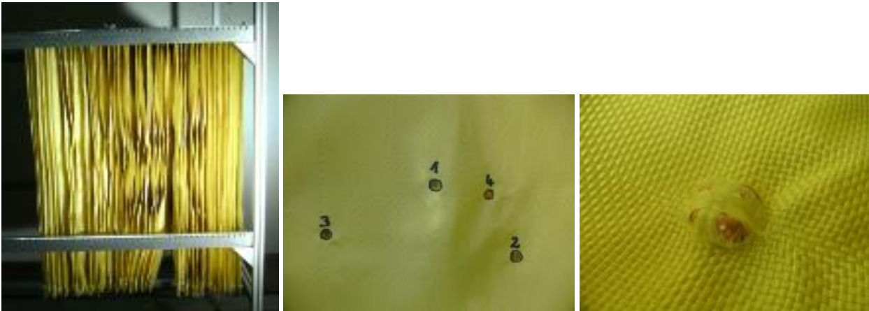
Figure 16: Aramid loose hanging right hand panama weaved Aramid which stopped a projectile
