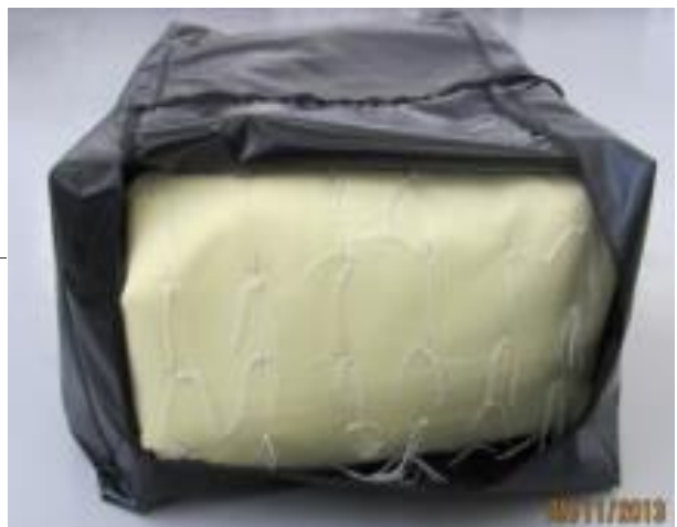
Figure 32: Inflatable frame of the demonstrator and the folded antiballistic pack integrated in a cover (transport box)
