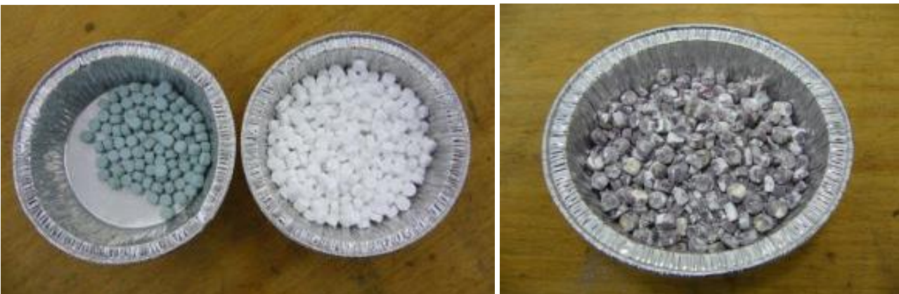
Figure 23: Fresh RAPTOR propellant in tablet geometry and fresh cooling agent (left: green: propellant, white: cooling agent); used cooling agent with slag residue on surface (right)
