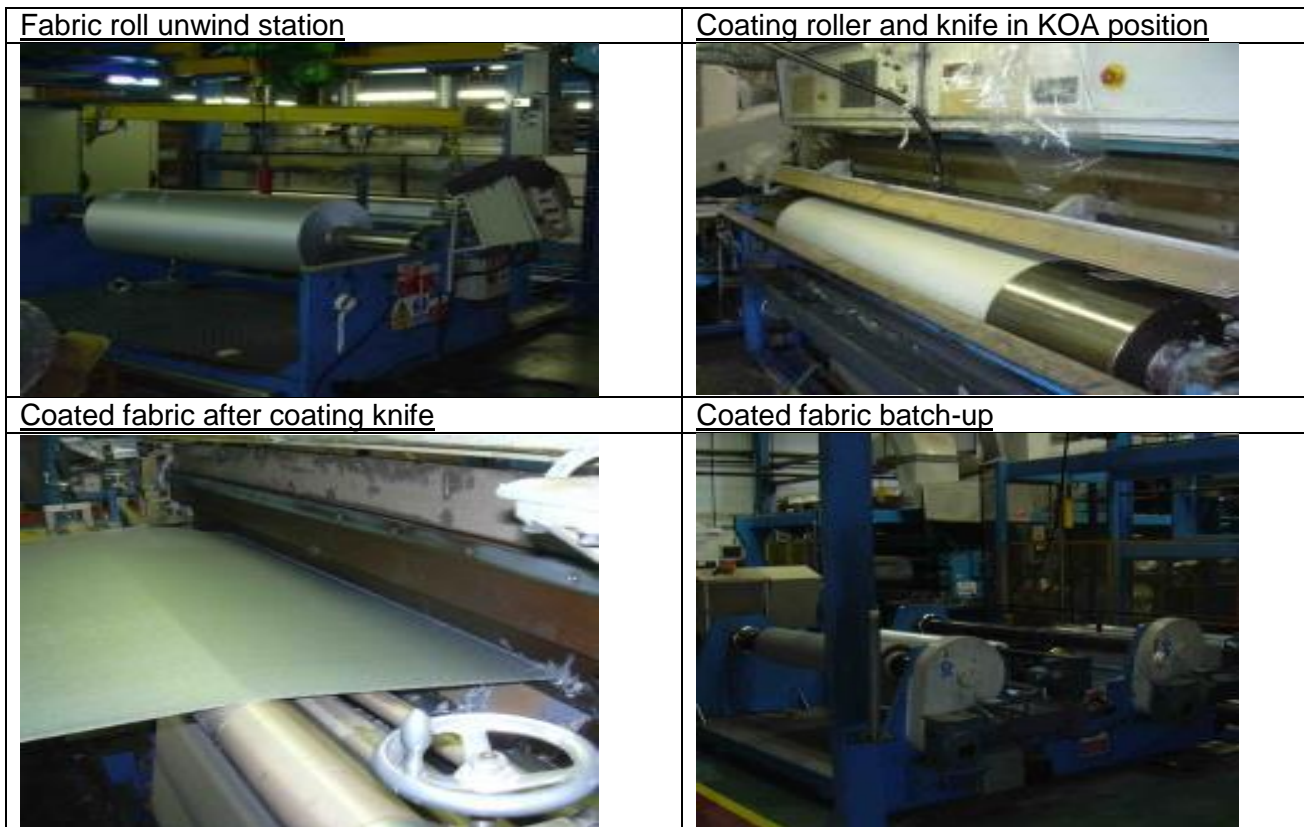
Figure 7: Photographs of Coating Line
