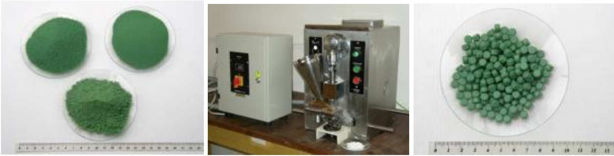
Figure 21: Process steps in gas generator processing
