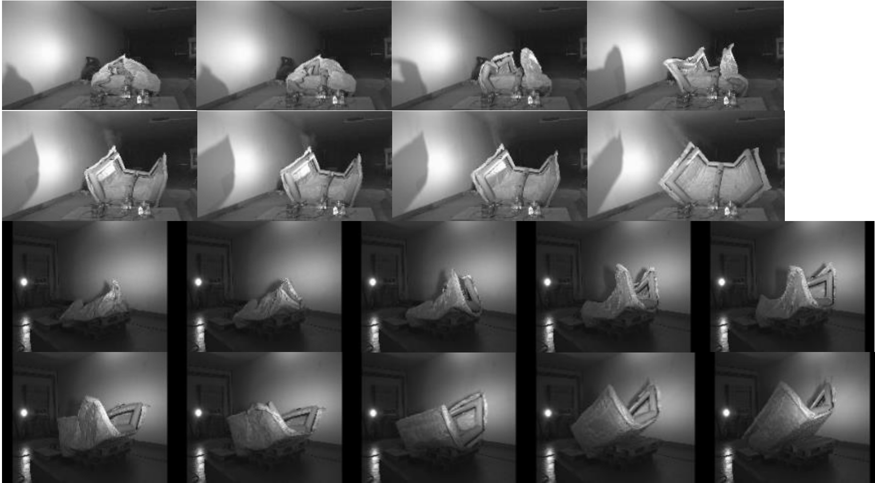
Figure 35: Sequence of a ballistic package when inflated by three cold gas generators as seen in Fig. 34, important steps of the deployment observed from head and back side
