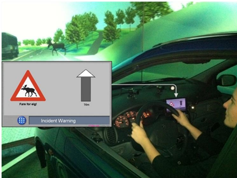
Figure: 15. The Incident and Hazard warning application shown in the driving simulator
