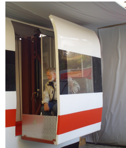
Cabin hoisting lift for the “long-distance and high-speed trains”
