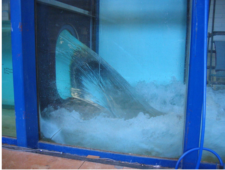
Figure 11 Flooding through a full-sized manhole in a flume tank tested in WP2/Task 2.3(Photo: Aalto University)
