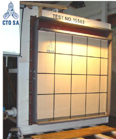
Figure 6 Test stand with a test specimen (in a frame) attached for the test in WP2/Task 2.1. In this case the test specimen is: cabin wall panel. (Photo: Deliverable D2.1b)
