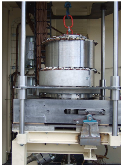
The 20 liters solvolysis reactor
