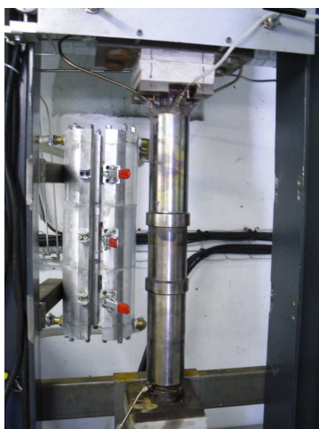
The 1 liter solvolysis reactor and cooling device
