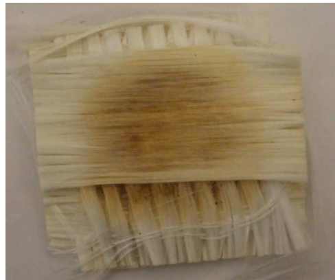
Evidence of diffusion, the resin is removed from the sides of the samples, not from the inside (50 x 50 mm).
