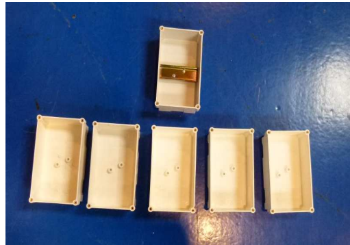
Prototypes of electrical boxes obtained with a EURECOMP BMC
