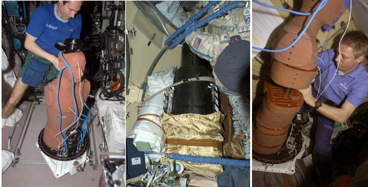
Figure Summary-2: MATROSHKA-2A: The MATROSHKA facility during the MATROSHKA-2A experiment phase (2006): (a) detector integration; (b) exposure inside the Russian PIRS module; (c) European astronaut Thomas Reiter removing the radiation detectors after the experiment for read out and data evaluation on ground.
