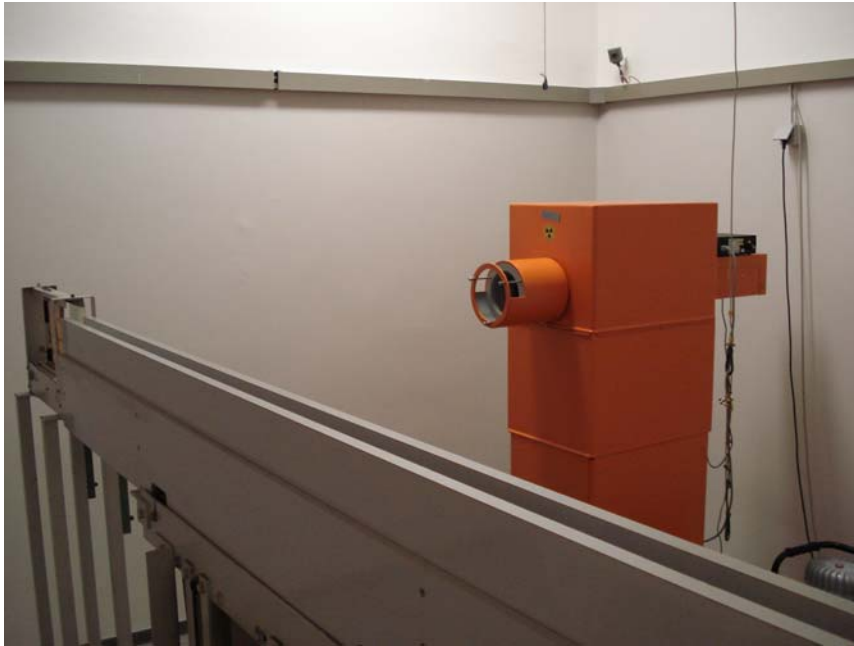
Figure WP2-6: TLD – Properties: (a) left part of the figure: Calibration stand of the Materialprüfungsamt (MPA), Dortmund, and (b) right part of the figure: Comparison of relative calibration factors for the applied thermoluminescence detectors used by the HAMLET partners in the frame of the experiment.
