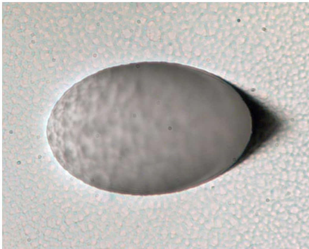
Figure WP2-4: CR-39: (a) left part of the figure: A microscopic picture of an iron ion passing through a CR-39 detector and (b) right part of the picture: the calibration curve (etch rate ratio vs. LET) for PNTD from IFJ, Krakow, Poland as measured for ions from HIMAC and GSI exposures.
