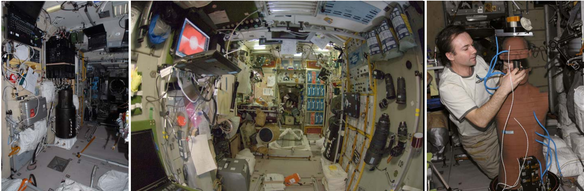
Figure Summary-3: MATROSHKA-2B: The MATROSHKA facility during the MATROSHKA-2B experiment phase: (a) and (b) exposure inside the Russian Zvezda module; (c) removal of the radiation detectors after the experiment for read out and data evaluation on ground.
