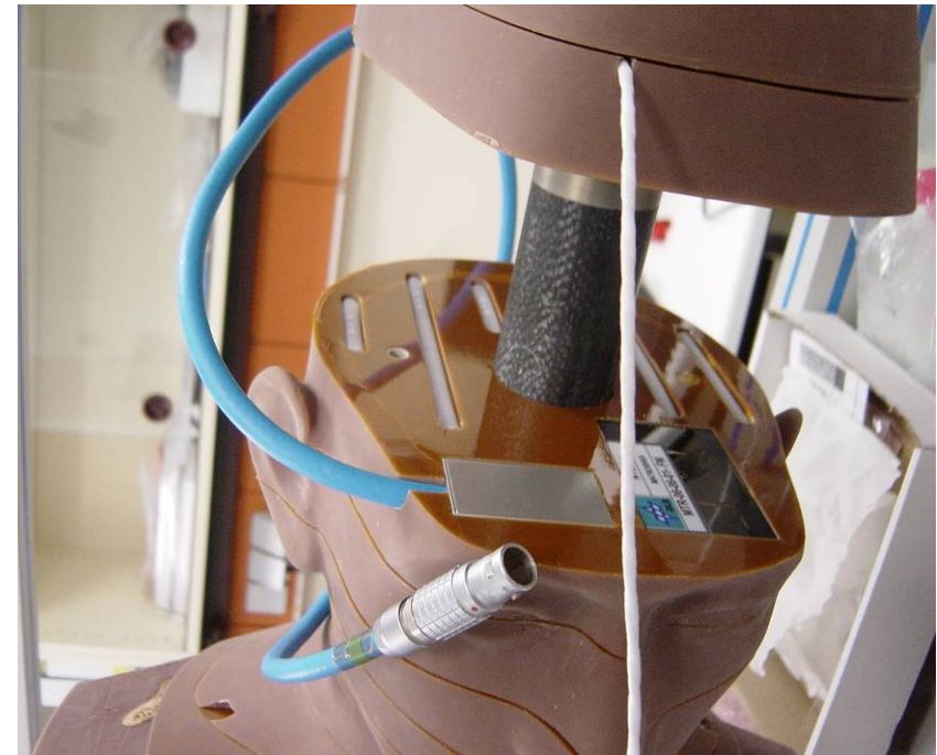
Figure Introduction-2: MATROSHKA-Detectors: View of the phantom upper torso (right) and the head (left) of MATROSHKA. It shows the phantom upper torso and the head of the phantom with the integrated passive and active radiation detectors. Passive detectors are integrated in polyethylene tubes and in the “organ dose” packages. The sensor for the active SSD instrument is shown with the blue cable connecting to the base structure. The white cable connects to a temperature sensor in the head of the phantom. Near the periphery, the outline of the skull can be perceived.
