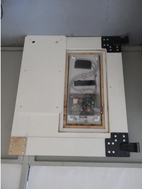
Isotrack Module installed in the prototype door
