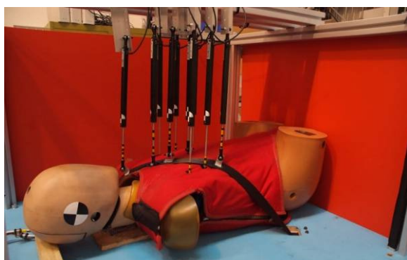
Fig. 21 Image of table top set-up with THOR-NT
