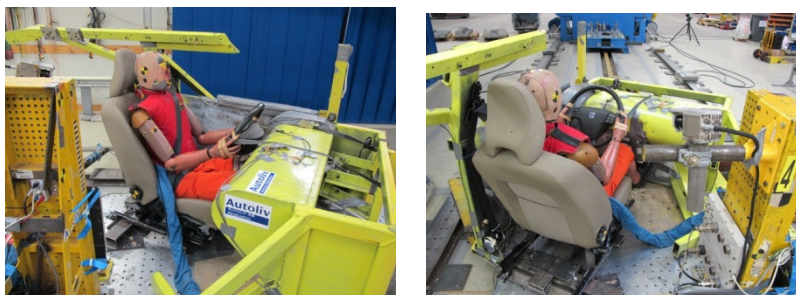
Fig. 34 Sled setup for 25° oblique with pre-deformed lateral intrusion
