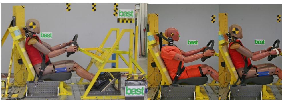
Fig. 32 Generic sled set-up used in the sled test at BAST
