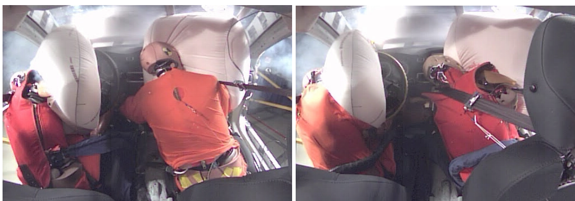
Fig. 35 BiW sled test at Euro NCAP pulse in 25° Oblique. To the left THOR is the driver and HIII the passenger. To the right THOR is the passenger and HIII the driver.
