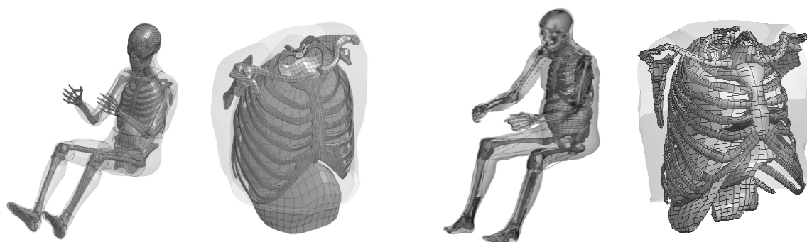
Fig. 6. Thorax part of the THOR (left) and HUMOS (right). Some parts have been hidden to facilitate visualization.
