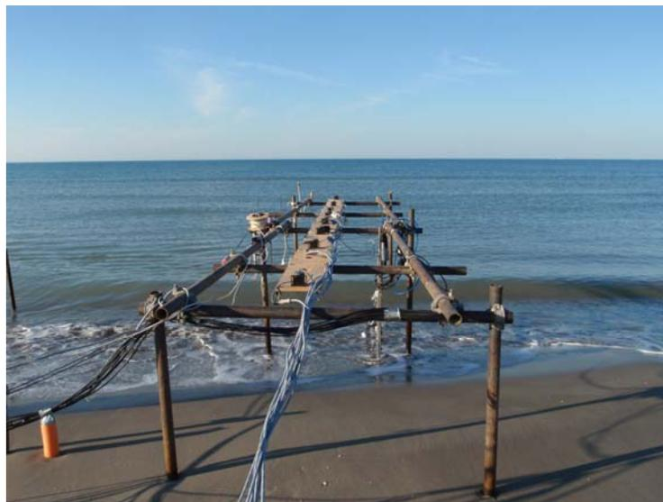
**Photograph 1** Cross-shore array of pressure sensors, velocimeters and ultrasonic devices deployed as part of work package 2 to study swash – groundwater interactions on a low-energy, microtidal beach. The ultrasonic devices have provided a unique insight into the response of the bed level to individual swash events.
