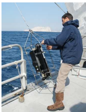
Fig. 1. LOPC–CTD–fluorometer on the RV Antedon in the Marseille Bay (Mar 29, 2009)
