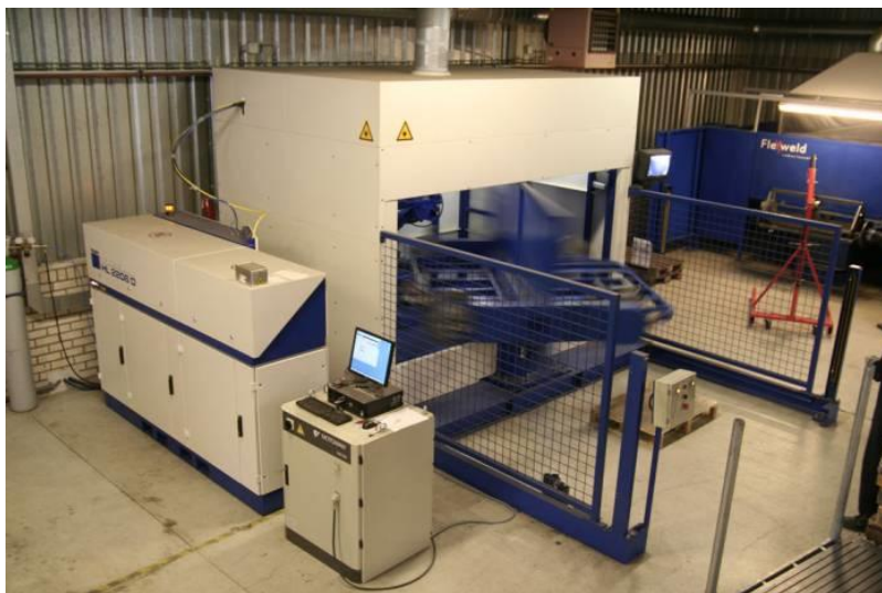
Figure 13: Laser welding installation in Flexweld b.v.
