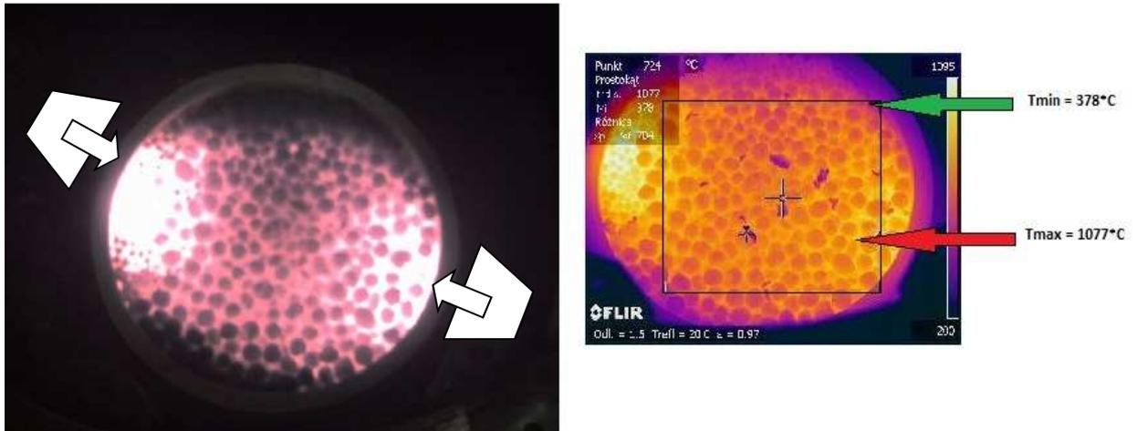
Photo 5. Distribution of temperature in the chamber of the MOS reactor.
