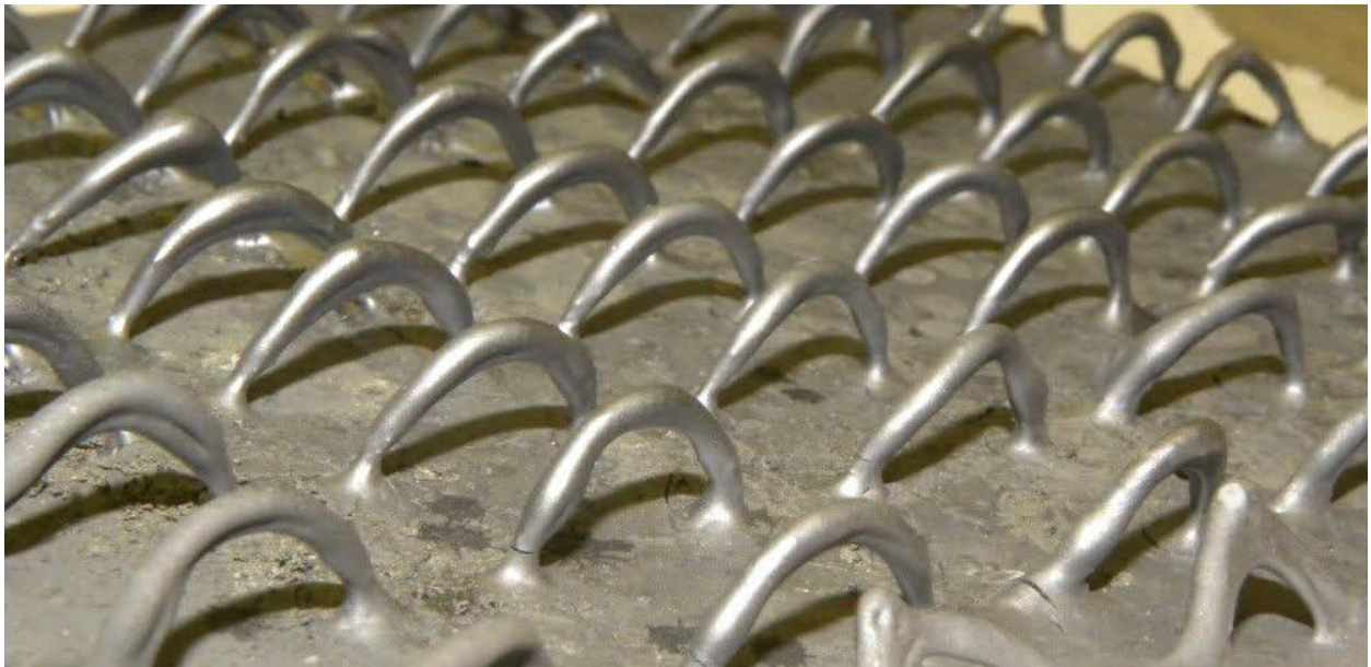
Figure 11: Si infiltrated SiC structure with loops as heat enhancing elements
