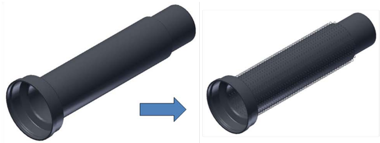
Figure 13: Model of the unstructured recuperative element left and with loops structured recuperative element right
