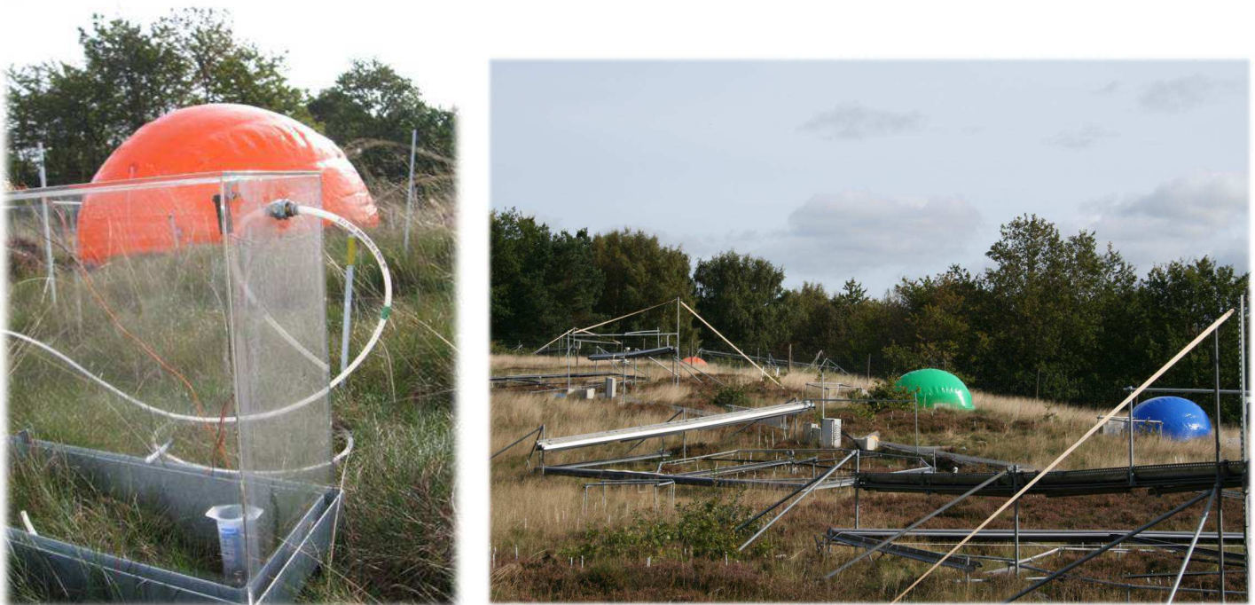
Figure 12. Set-up of the ^{13}\text{C} pulse-labelling experiment at Brandbjerg, Denmark. Ballons contained ^{13}\text{C} labelled air in ambient and elevated \text{CO}_2 concentration (510 ppm).
