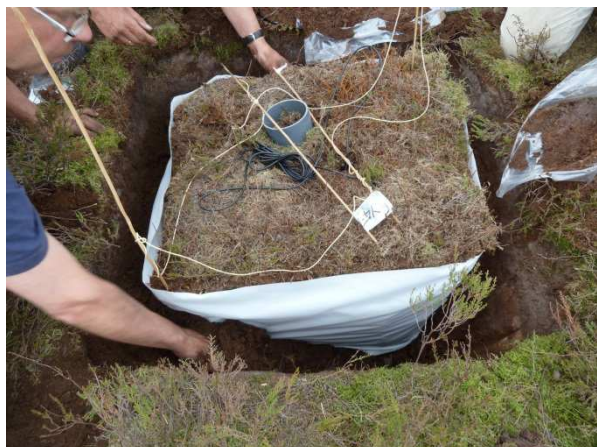
Figure 10. Preparing (15 cm wide, 45 cm deep) trenched plots of 60 by 60 cm, at Oldebroek.
