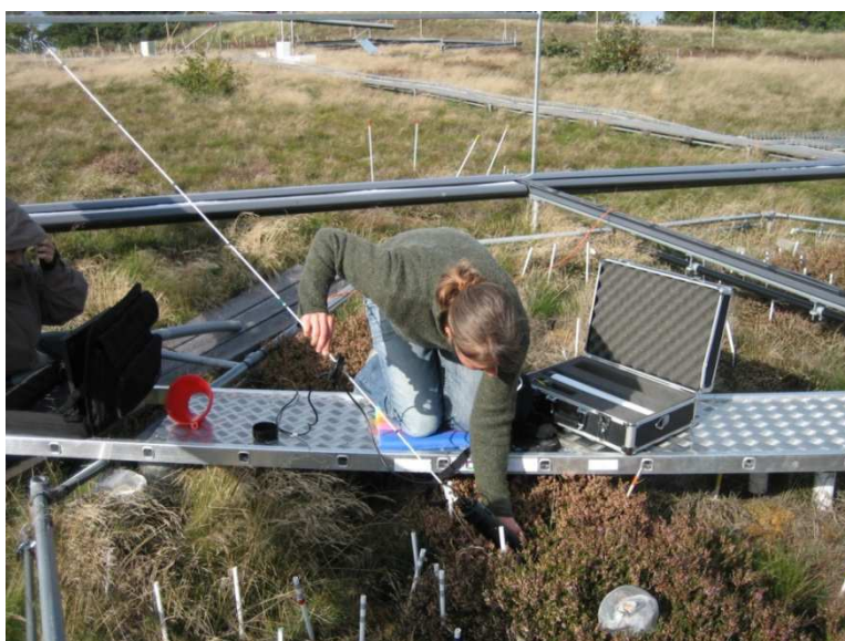
Figure 11. Scanning roots within the minirhizotrons at Brandbjerg.
