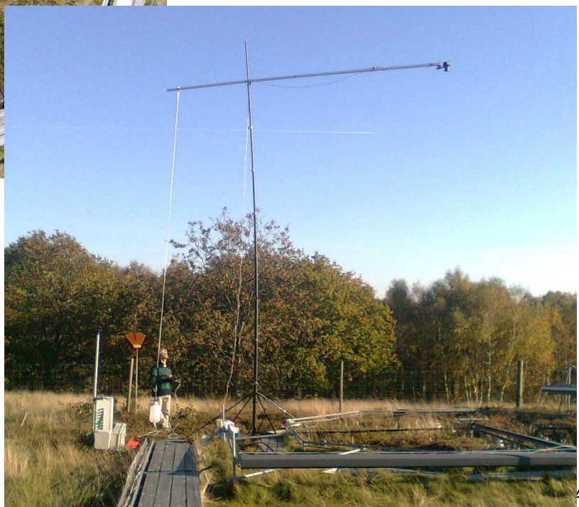
Figure 5: Telescope pole set-up for aerial photography .
