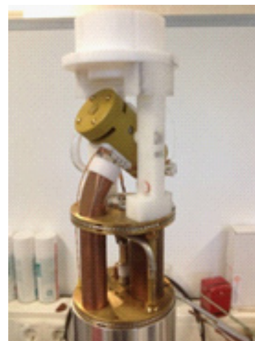
Low temperature DNP MAS probe with THz excitation waveguide.
