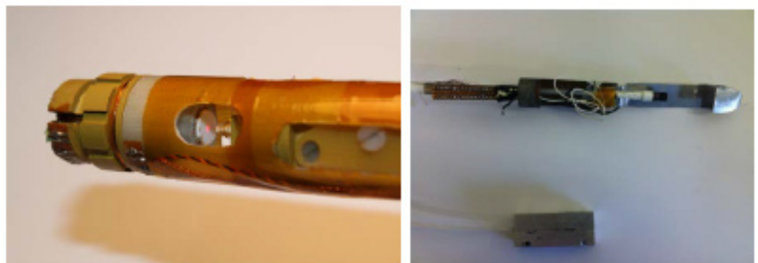
Figure 3: Left panel: Lower part of the insert for photoconductivity experiments in pulsed field magnets at the LNCMI – Toulouse. Right panel: Lower part of the insert for photoconductivity experiments in DC field magnets at the LNCMI – Grenoble.
