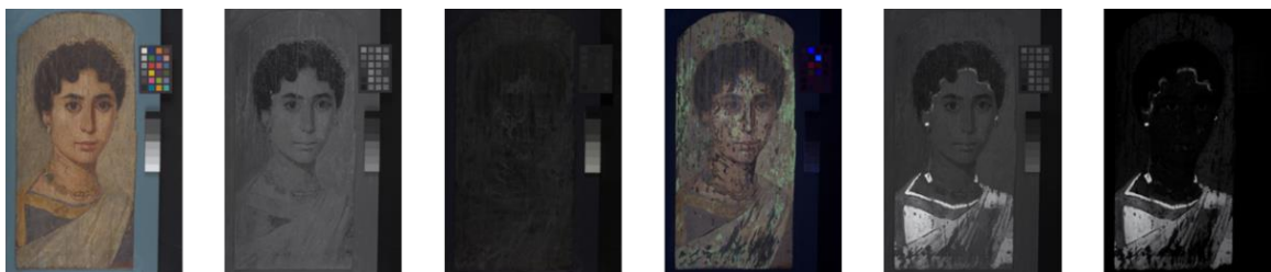
Fig. 3.4.8 (from left) Visible- (VIS), IR- (IRR) and UV-reflectance (UVR), UV-induced visible luminescence (UVL) and two visible-induced IR luminescence (VIL) images of a Fayum portrait from the British Museum.
