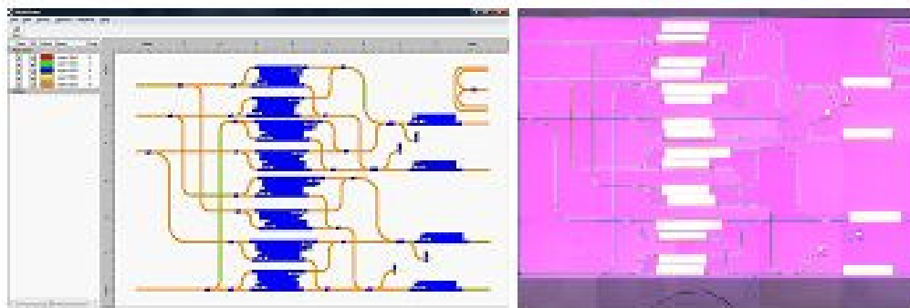
Figure 6 An example of what can be achieved with the design kit; the left half of the figure shows the mask level information, the manufactured die is photographed on the right (Design: University of Cambridge, Fab: Oclaro. See Proc OFC 2012 for more details)
