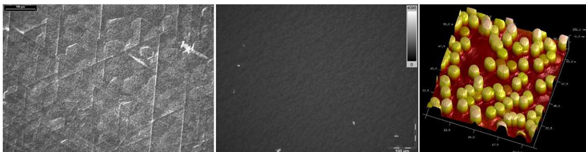
Figure 5.6: Left: Normaski microscopy image of NAV_00928 showing a high amount of cracks. Middle: Normaski microscopy image of NAV_00942 without cracks due to improved strain management. Right: 100µmx100µm AFM scan of the initial surface showing circular features of > 200nm height, which could be overgrown.
