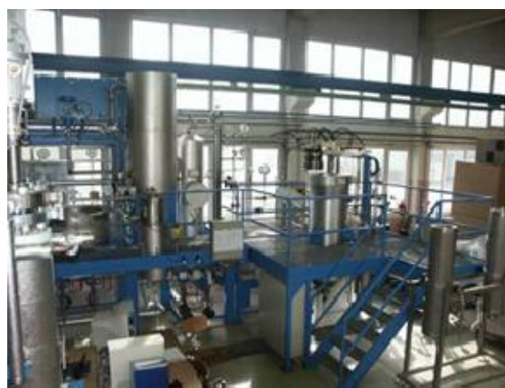
Figure 6 Example of the extraction yields in scaling up the scCO 2 extraction of triterpenic acids (TTAs) from eucalyptus outer bark and 80L/550bar pilot plant in NATEX laboratory Hardwood bark as a source of valuable components
