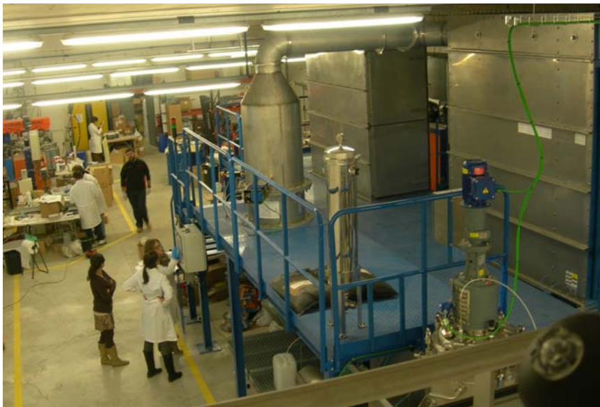
Figure 6. Industrial FSP line with 5 kg/h production
